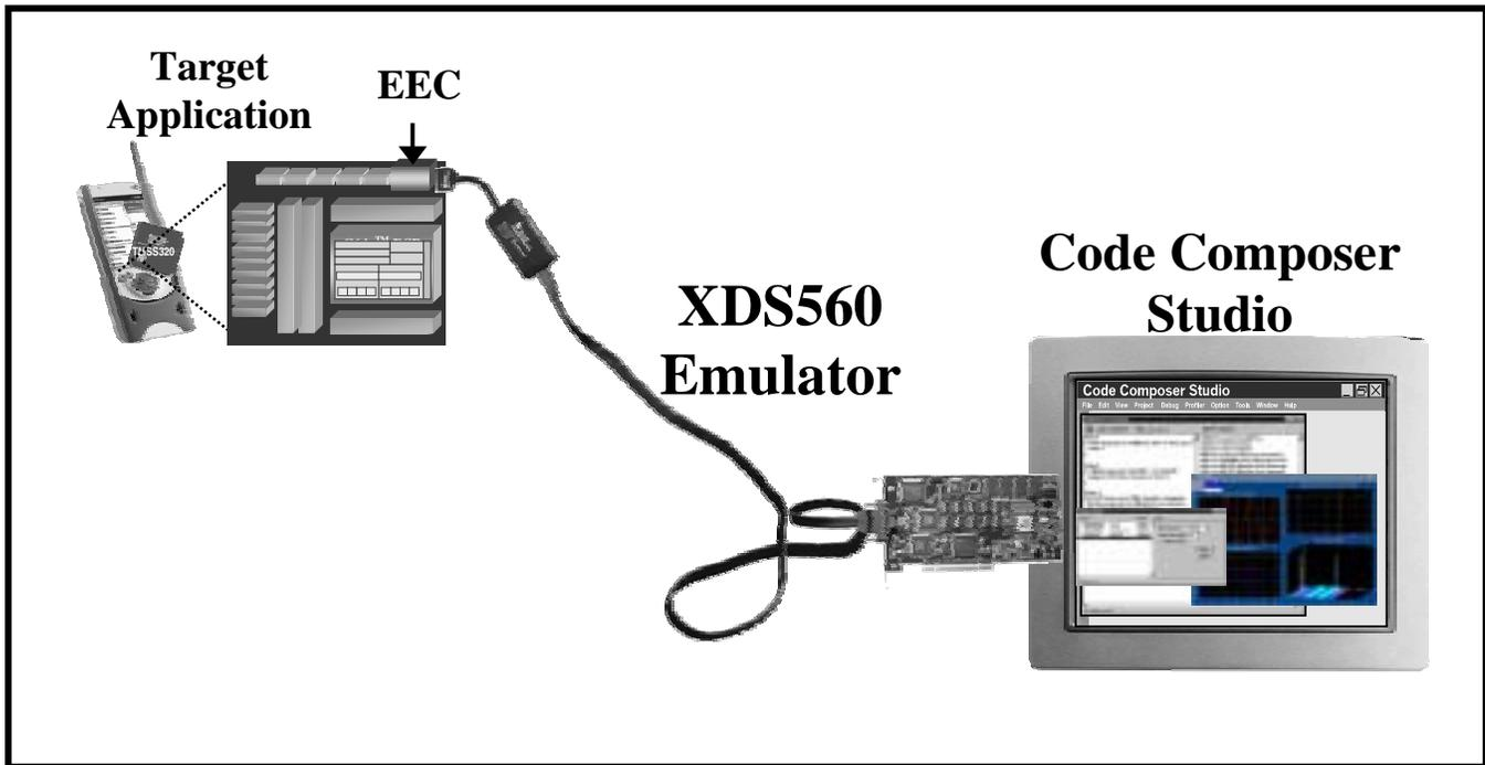
This application note provides a guided tour of the advanced event triggering capability available with TI's TMS320C6211™ DSP generation and TMS320C6711™ generation digital signal processor chips, the XDS510/XDS560 emulator, and Code Composer Studio version 2.0/2.1.
