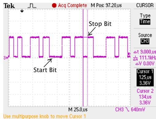
**Figure 15. Oscilloscope Capture**
