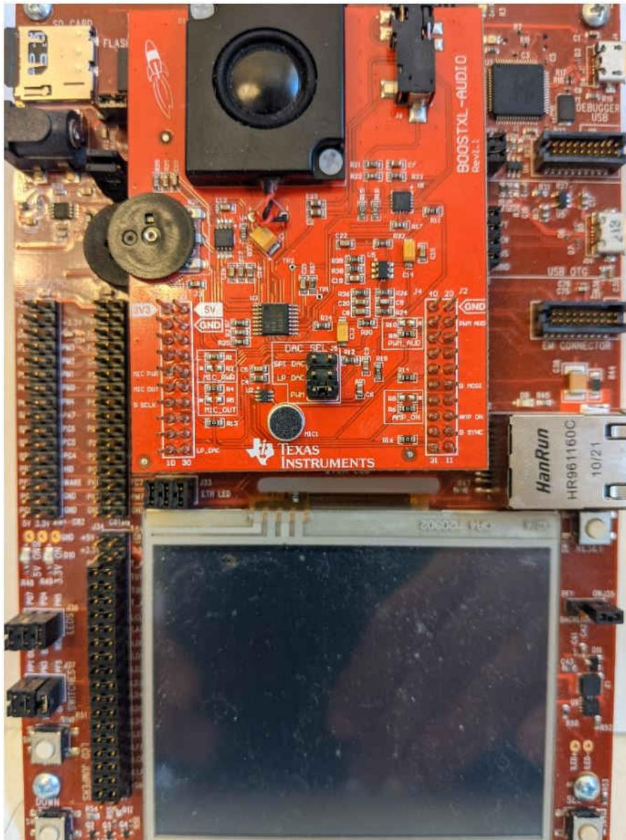
**Figure 5-4. EK-TM4C129x Development Board With Audio BoosterPack**
