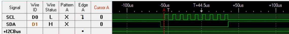
Figure 10. I2C Transaction for I2C\_MASTER\_CMD\_BURST\_SEND\_CONT
