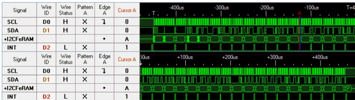
Figure 17. Receive With CPU and Non FIFO
