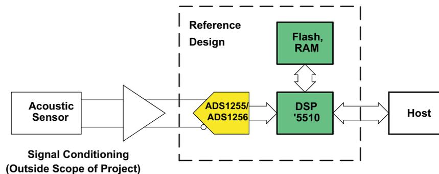
**Figure 1. Seismic System Architecture**
