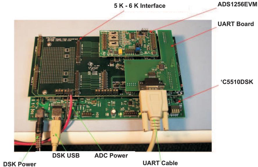
**Figure 4. Seismic System Prototype Board**
