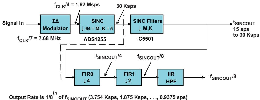
Figure 3. Filtering Architecture Block Diagram
