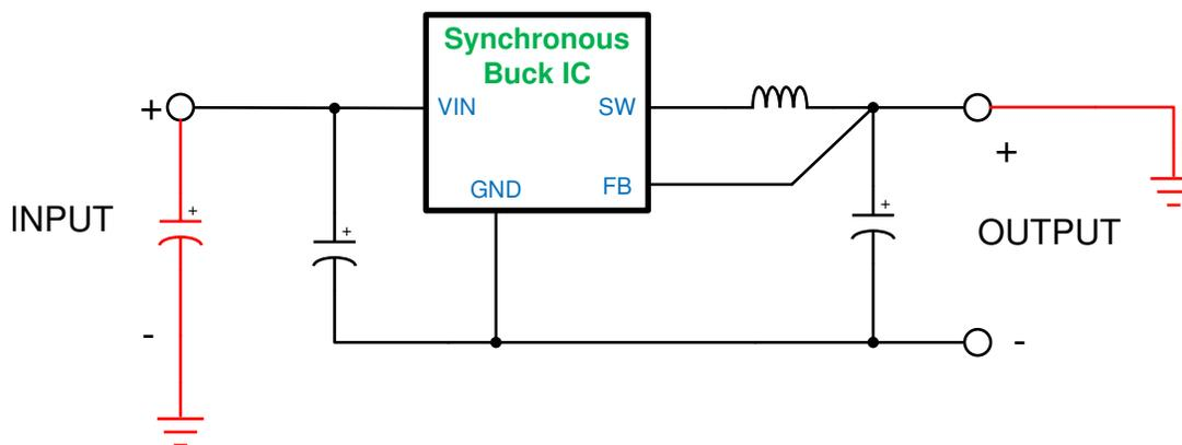
Figure 2. Converting a Buck to an Inverting Buck-Boost
