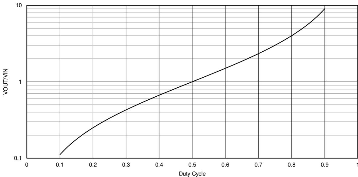
Figure 4. Conversion Ratio vs Duty Cycle
