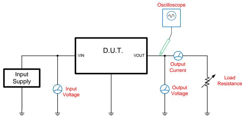
Figure 5. Current Limit Test Setup
