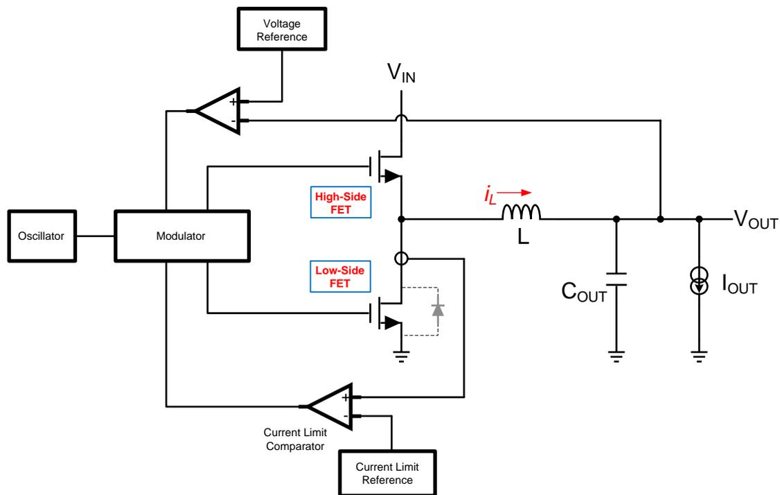
Figure 8. Synchronous Buck Converter with Valley Current Limit
