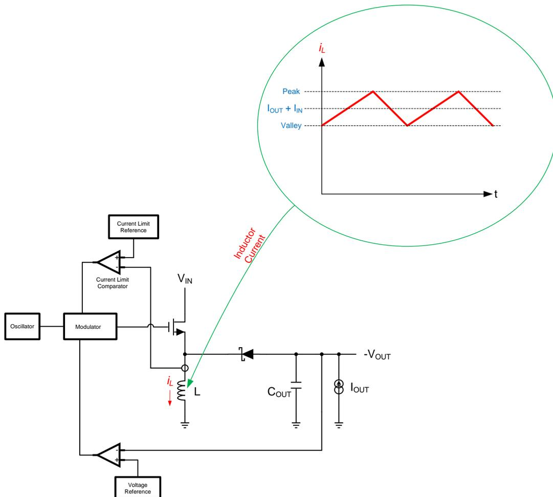
**Figure 11. Simple Inverting Regulator**
