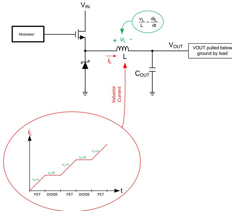
Figure 9. Negative Output Voltage Conditions
