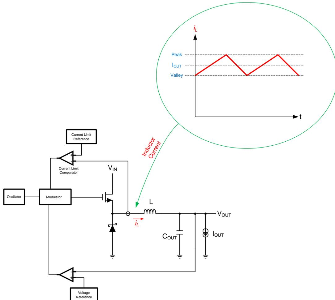
Figure 6. Simple Buck Converter
