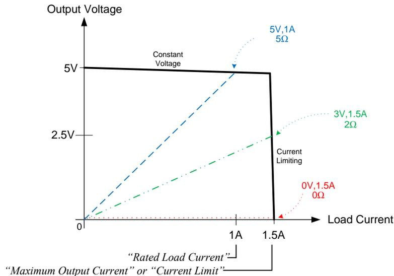
Figure 1. Brick-wall Current Limit Profile
