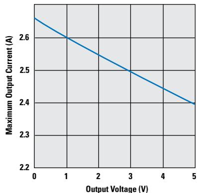
**Figure 5. Maximum Output Current vs Output Voltage**
