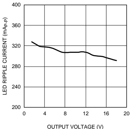
Figure 2. Ripple Current vs. Output Voltage
