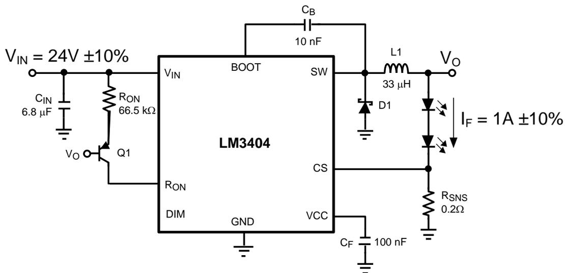
**Figure 1. Constant Ripple LED Driver Using the LM3404 Buck Regulator**
