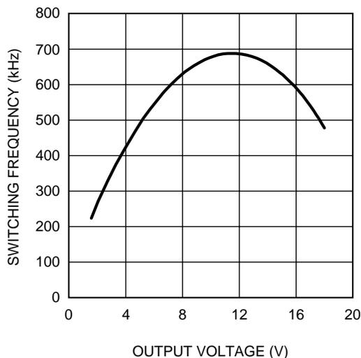
Figure 3. Switching Frequency vs. Output Voltage
