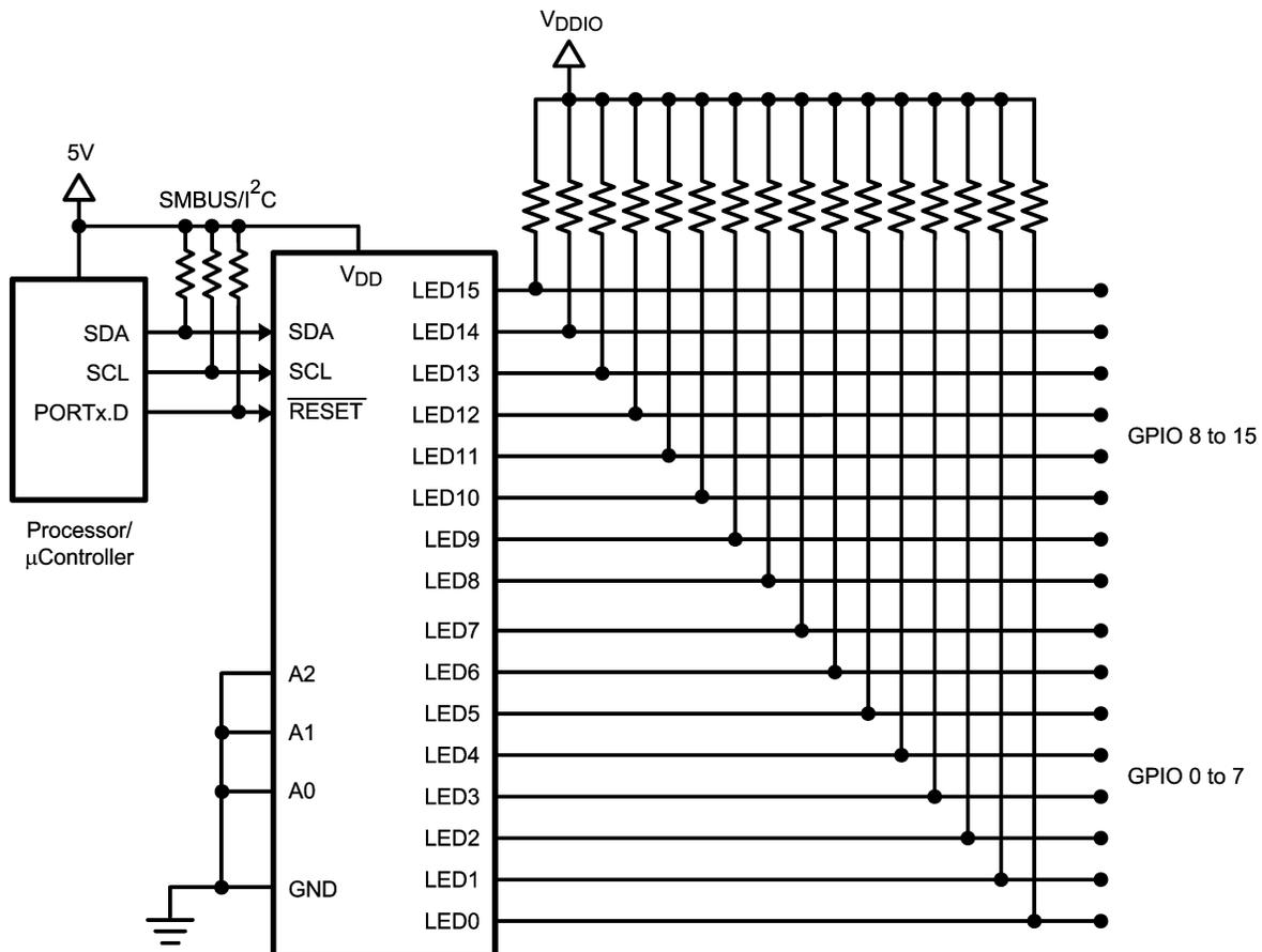
Figure 1. LP3943 Configured to 16 Channel GPIO Expander
