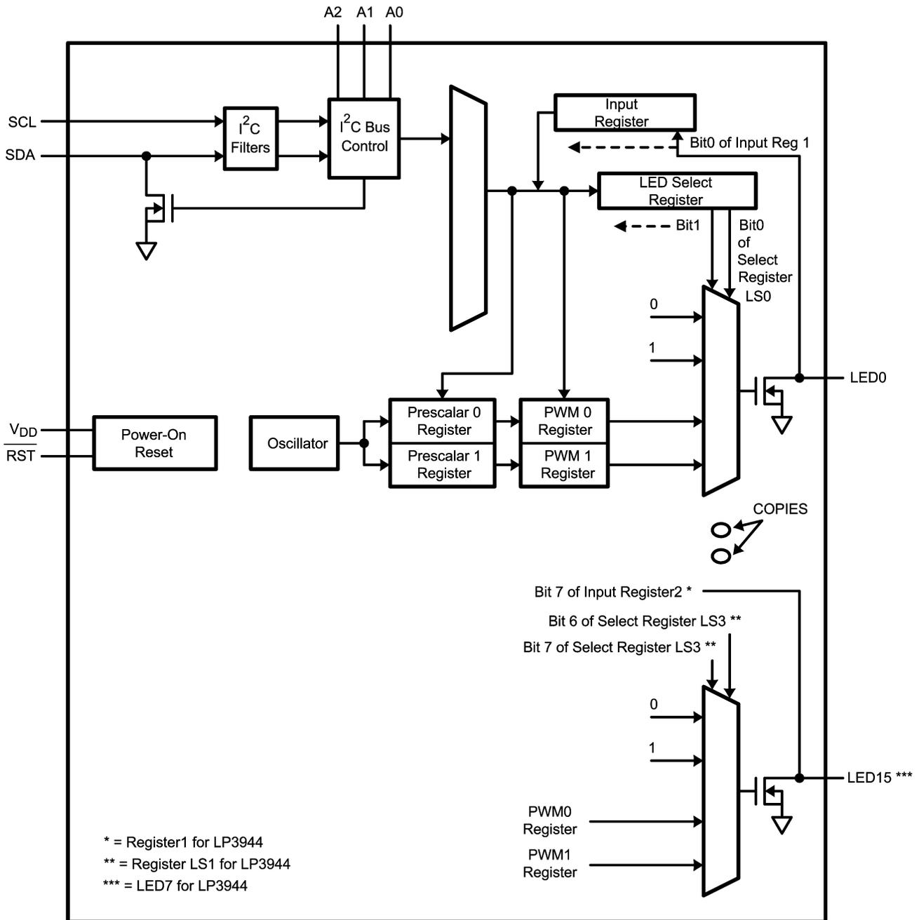
Figure 2. LP3943/44 Block Diagram
