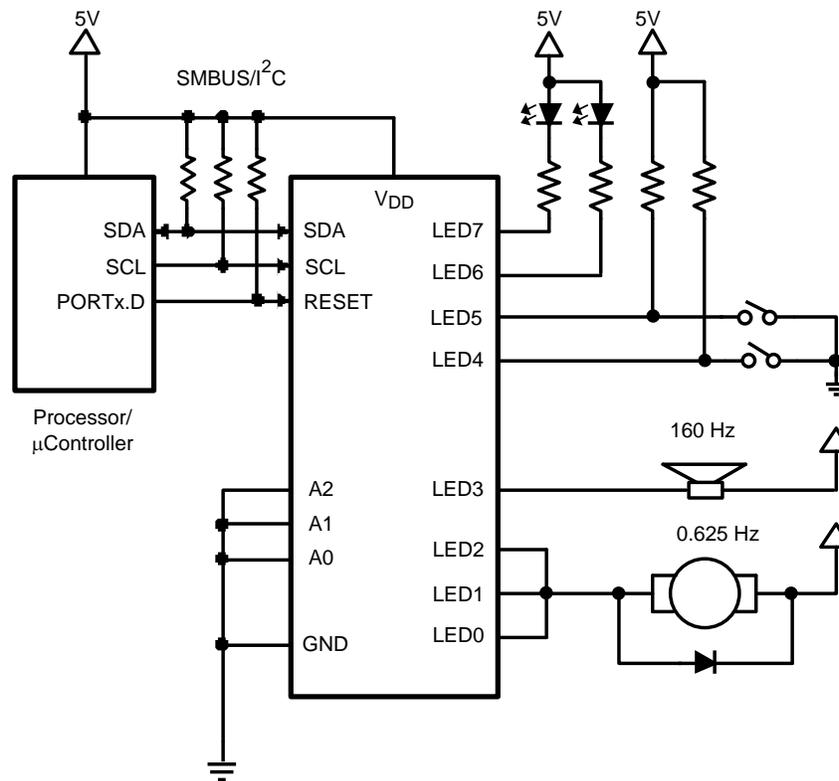
**Figure 3. LP3944 in Mixed Mode Configuration**
