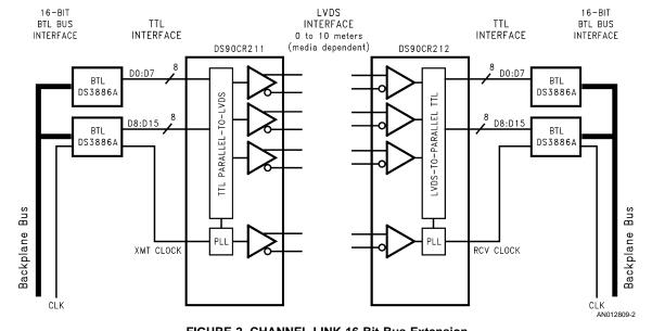
FIGURE 2. CHANNEL LINK 16-Bit Bus Extension
