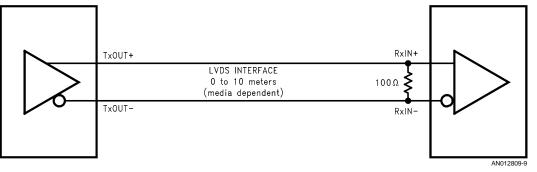
FIGURE 9. LVDS Serialized Link Termination
