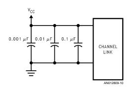
FIGURE 10. CHANNEL LINK Decoupling Configuration
