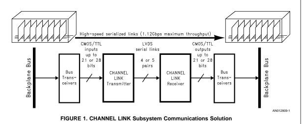
CHANNEL LINK is a low power means of transporting high-speed data over an interconnect. LVDS technology represents a significant decrease in power to comparable high-speed transmission devices such as PECL. The CHANNEL LINK transmitter has a dynamic loaded Icc of 35 mA (typical) while the CHANNEL LINK receiver is 60 mA (typical). CHANNEL LINK also includes a Powerdown mode which reduces total device power to < 5  $\mu$ W (typical).
