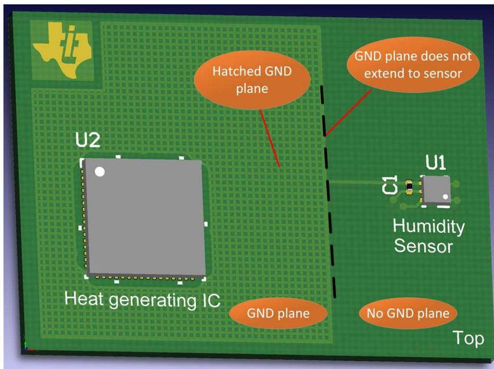
**Figure 10. GND Plane Does Not Extend To Sensor**
