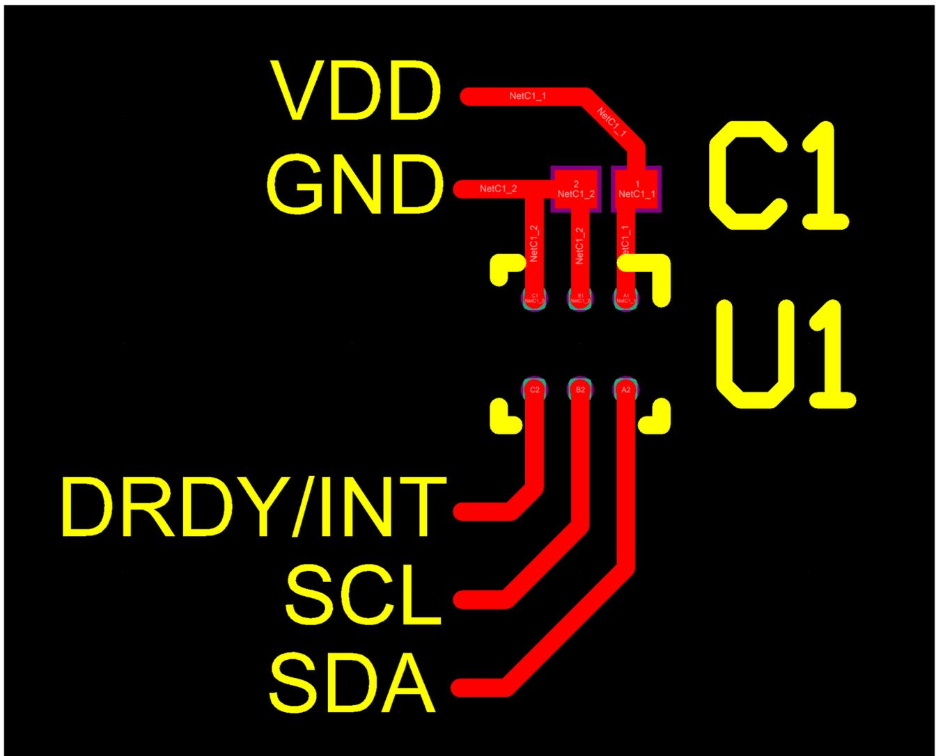
Figure 17. PCB Layout Example HDC1010, HDC2010 [DSBGA Package]
