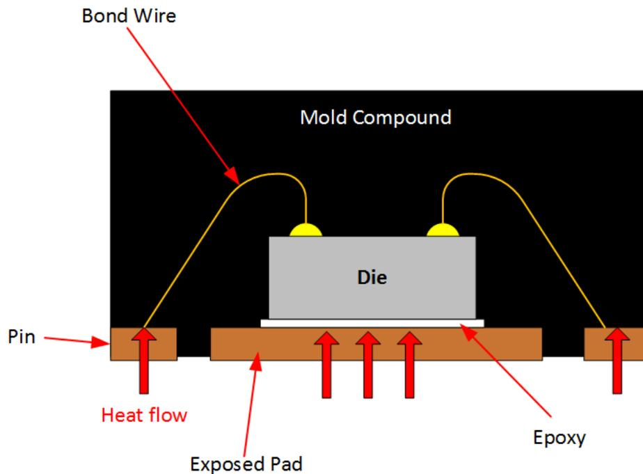
Figure 20. Heat Transfer WSON (HDC1080[DMB]) Package Cross Section
