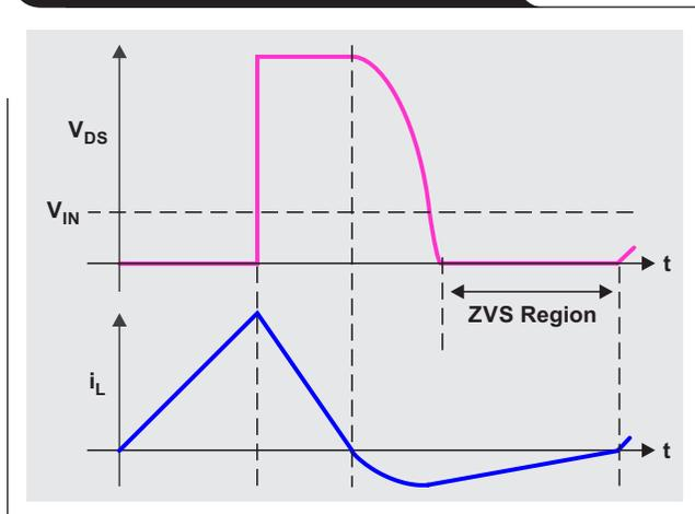
Since the MOSFET turns on when the inductor current reduces to zero, the PFC now works as if it is in critical conduction mode (CrM). The switching frequency is not constant any more—it increases. ZVS significantly reduces switching losses and improves efficiency.
