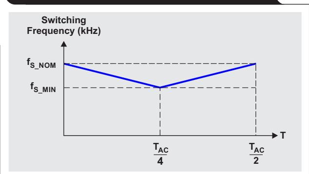
The frequency dithering is not the same as the widely used spread-spectrum frequency dithering technique to reduce electromagnetic interference (EMI) noise. In that technique, the switching frequency is swept back and forth around the nominal value. Because the average switching frequency does not change, the average efficiency is not improved.
