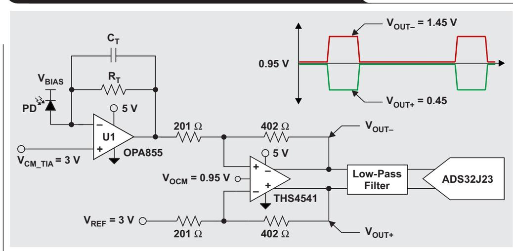
To recover the lost ADC bit, the THS4541 can be configured such that under no-light conditions, its individual outputs are offset so as to produce a negative full-scale output from the ADC32J23, as shown in Figure 7. Under these conditions, the output of the THS4541 now has 2x the linear swing range compared to Figure 6, thus improving the signal-to-noise ratio (SNR) of the system by 6 dB.
