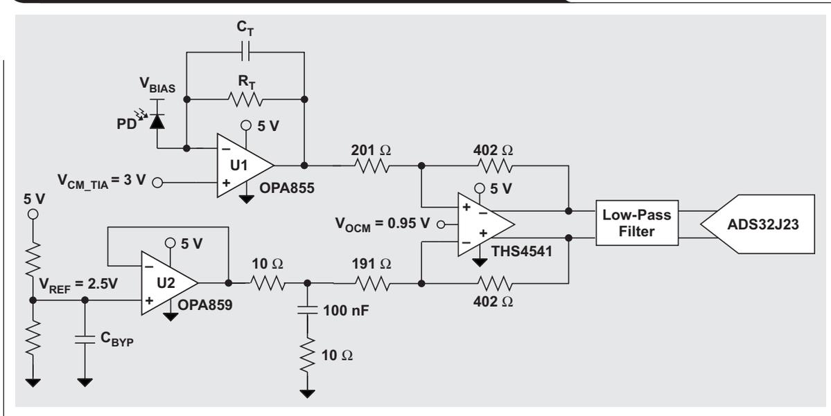
**Figure 9. DC offset circuit with AC coupling between the TIA and the differential-amplifier**
