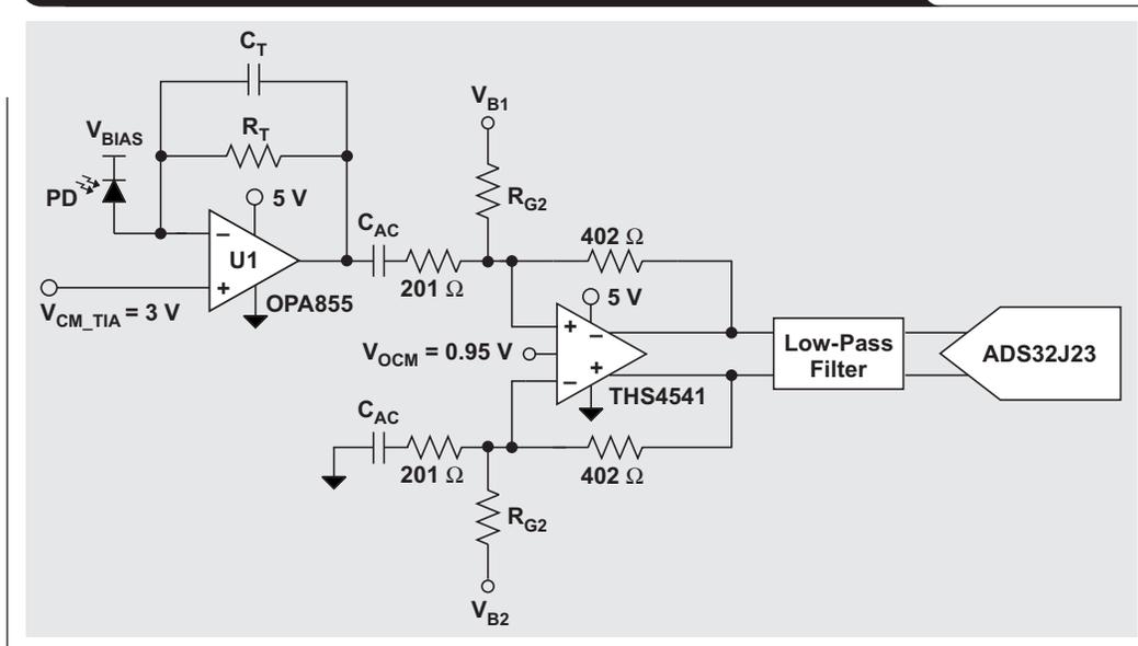
The  $V_{B1}$  and  $V_{B2}$  voltages can usually be set to the supply voltage and ground respectively, and adjust  $R_{G2}$  accordingly to create the specified DC offset. For example, if  $V_{B1} = V_{CC} = 5\text{ V}$  and  $V_{B2} = 0\text{ V}$ , then  $R_{G2}$  can be calculated.
