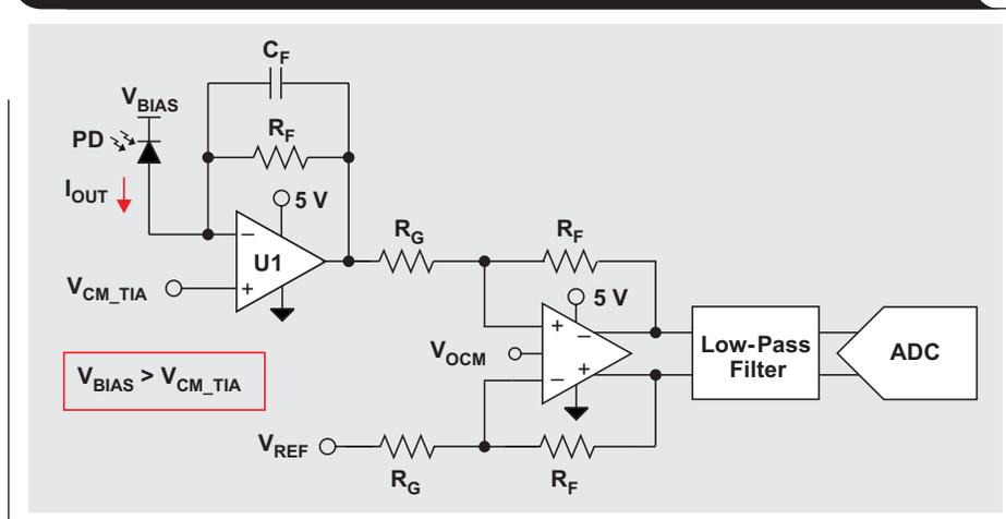
**Figure 2. Analog front-end for optical signal chain with anode bias**
