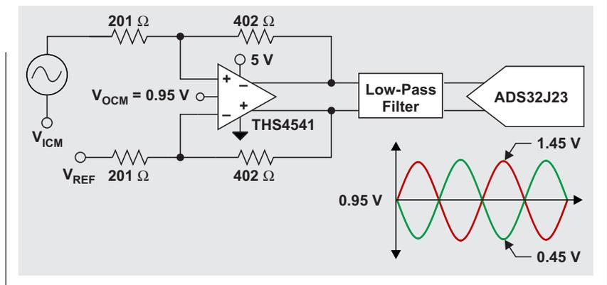
Figure 6. Signal-chain performance with  $V_{CM\_TIA} = V_{REF}$
