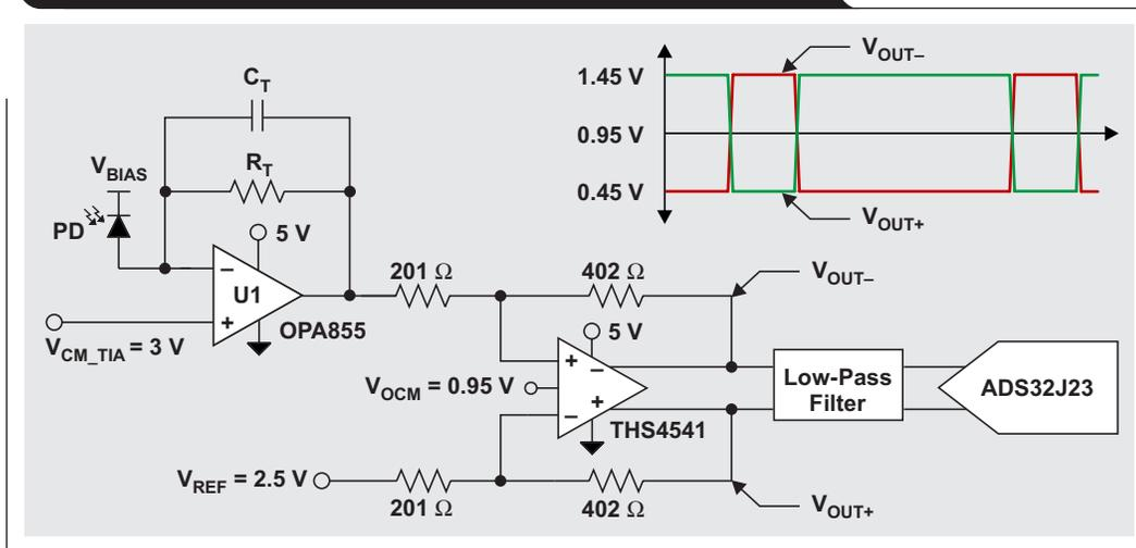
To save power, an amplifier with lower bandwidth can be used to set the DC bias. However, to ensure low impedance across frequency, it's best to use an AC bypass capacitor, as shown in Figure 8. Since most operational amplifiers cannot directly drive large capacitors, a series isolation resistor will be required to maintain stability. The circuit shown in Figure 8 ensures stability and balance.
