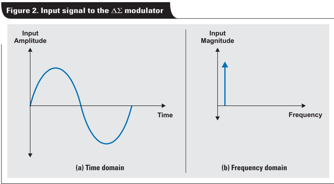
Figure 2a shows a single cycle of a sine wave for the input of a  $\Delta\Sigma$  modulator. This single cycle has voltage amplitude that changes with time. Figure 2b shows a frequency-domain representation of the time-domain signal in Figure 2a. The curve in Figure 2b represents the continuous sine wave in Figure 2a and appears as a straight line or a spur.
