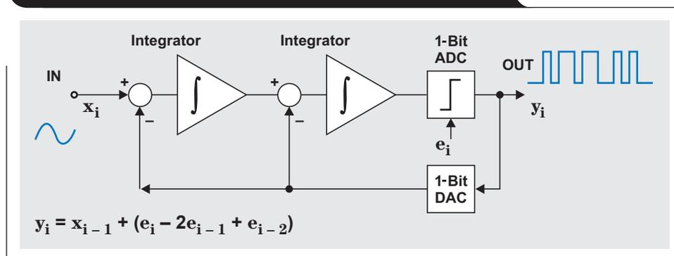
and increased design difficulty. However, most  $\Delta\Sigma$  modulators are higher-order, like the one in Figure 5. For instance, Texas Instruments  $\Delta\Sigma$  converters include second- through sixth-order modulators.
