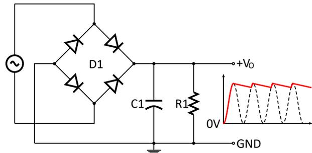
Figure 1. Classic Full-Wave Diode Bridge DC Rectifier
