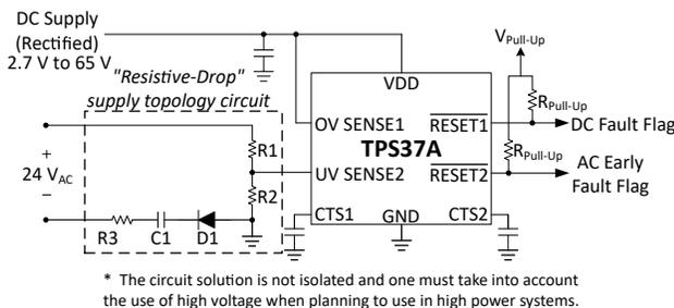
**Figure 2. Half-Wave AC Circuit on UV SENSE2 Input**
