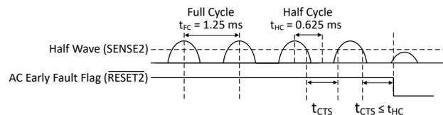
**Figure 3. Timing Diagram**
