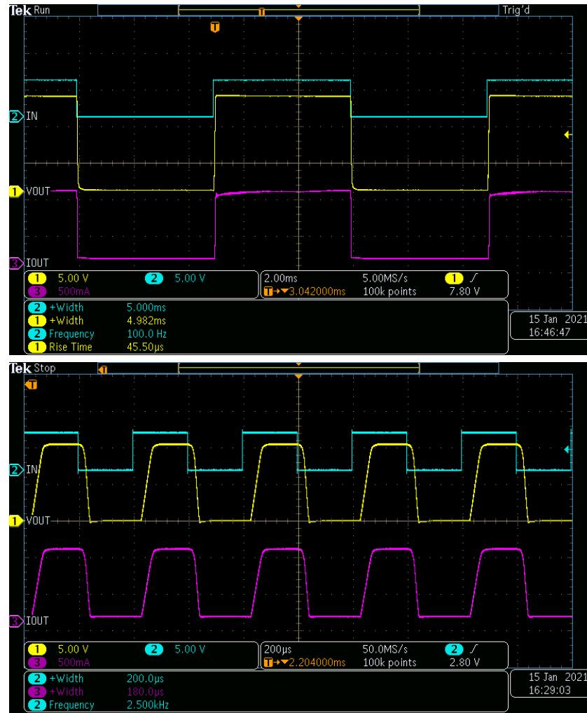
**Figure 3-1. Switching Too Fast in a TPS1H000-Q1 Resistive Load Setup**
