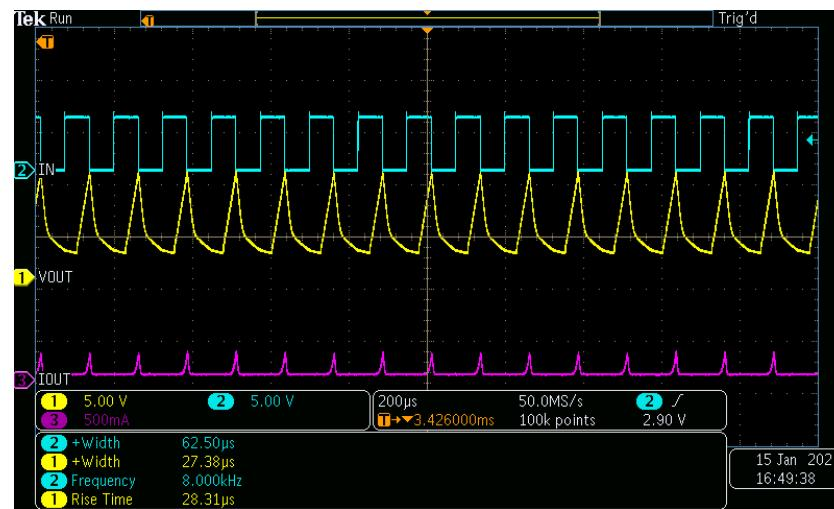
**Figure 3-15. Bench Results of 12-V, 500-mA PWM Diode Load Over Frequency**
