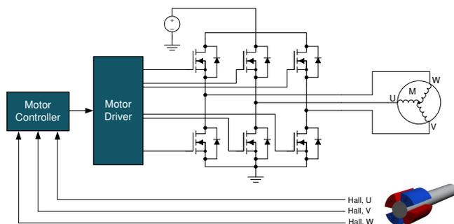
Figure 1. Closed-Loop System for BLDC Motor Control
