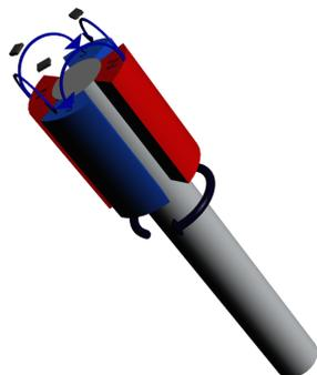
**Figure 5. Rotor Position Using Surface Mount Hall Sensor**
