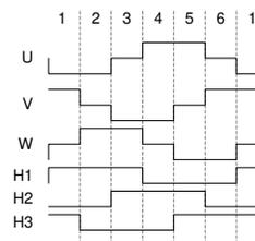
Figure 2. PWM Winding States (High, Low, Off) for U, V, or W in Relation to Hall Sensor Outputs for H1, H2, and H3
