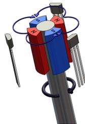
**Figure 4. Rotor Position Using TO-92 Hall Sensor**
