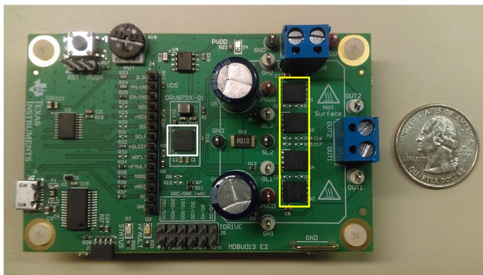
Figure 12. DRV8702-Q1EVM With MOSFETs and Motor Driver IC
