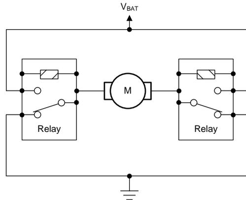
**Figure 3. H-Bridge Control of BDC Motor Using Relays**
