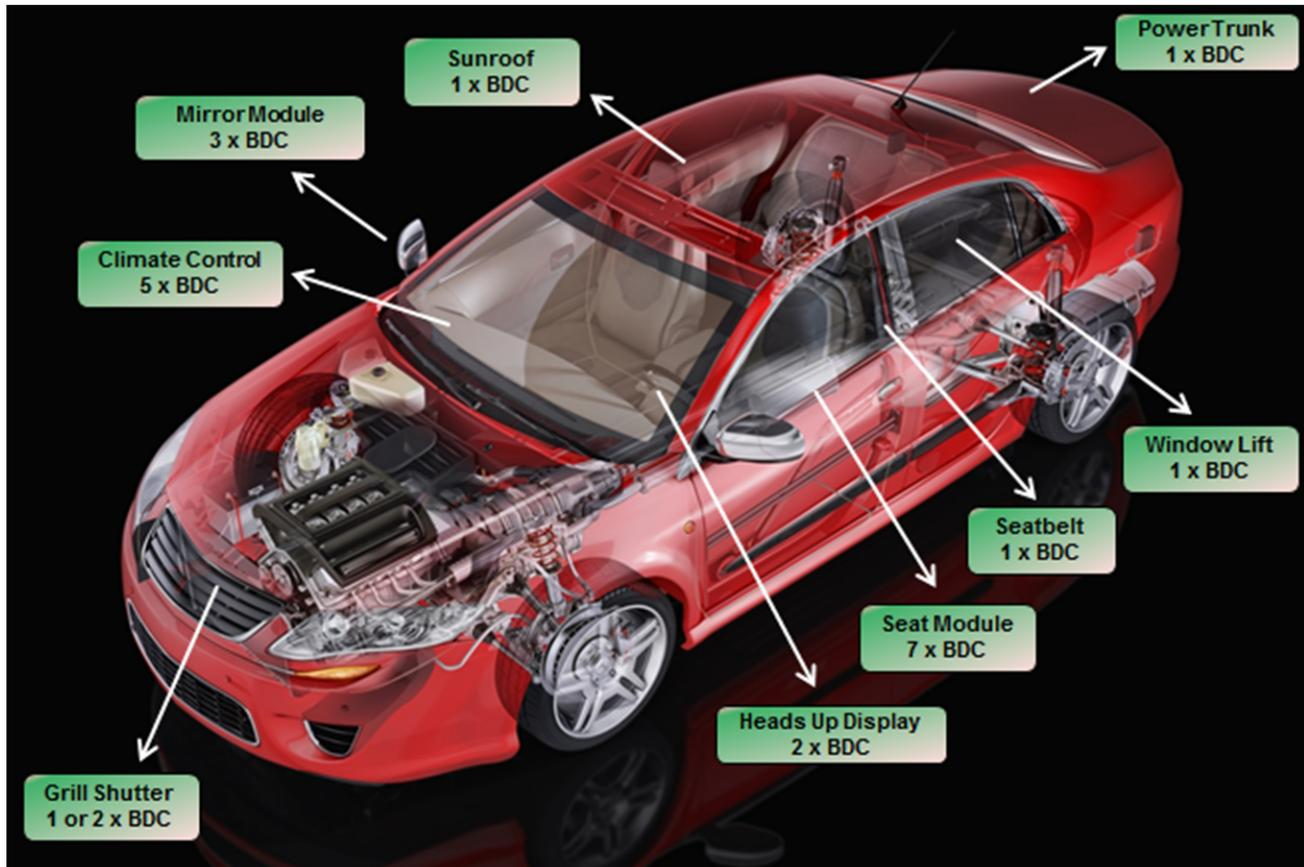
Figure 1. BDC Motor Applications in a Vehicle
