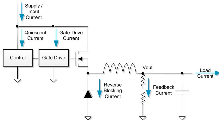
**Figure 1. Asynchronous Buck Converter and Associated Currents**
