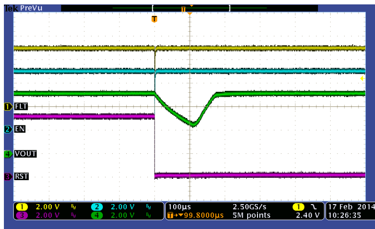
Figure 7. TPS7A63xx VOUT Response With 200-µs Time Units, I_o = 300 mA
