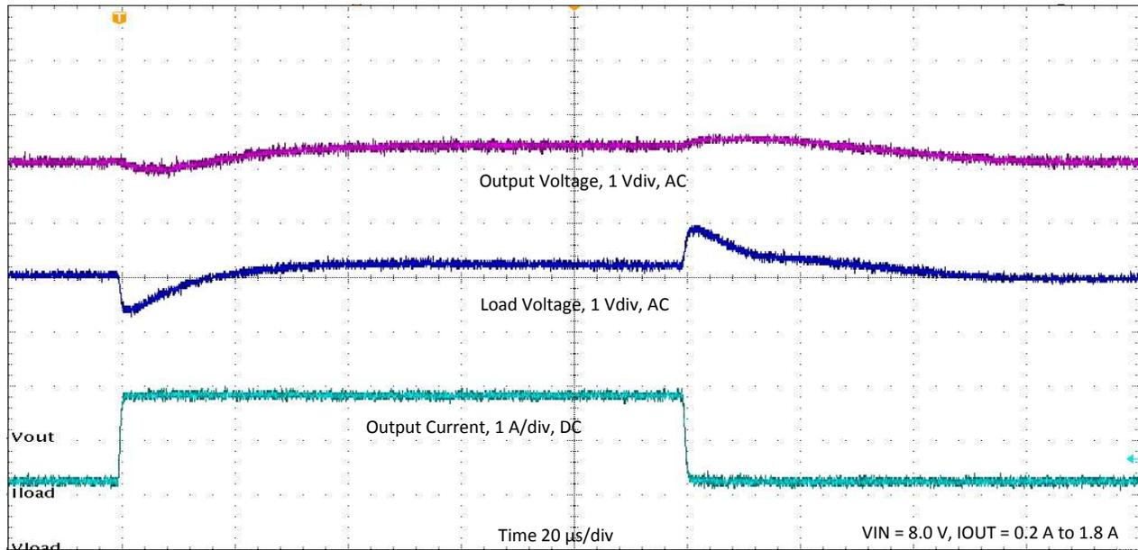
Figure 4. Load Transient
