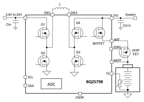
Figure 3-3. BQ25798 Fully Integrated Buck-Boost Charger
