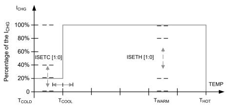
Figure 4-1. BQ25798 Charging Current Temperature Profile
