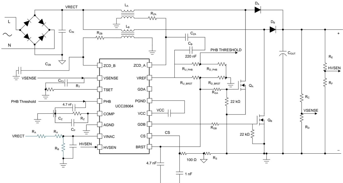
Figure 11. UCC28064A Application Schematic
