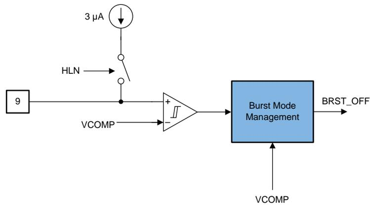
**Figure 8. Burst Mode Block Diagram**
