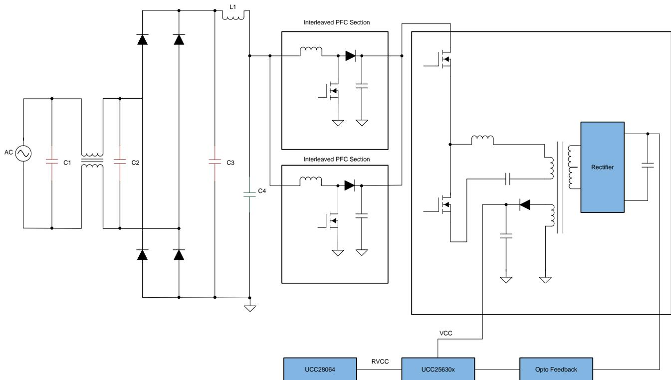
**Figure 7. Most of EMI Filter Capacitance to the Right of Bridge Rectifier**
