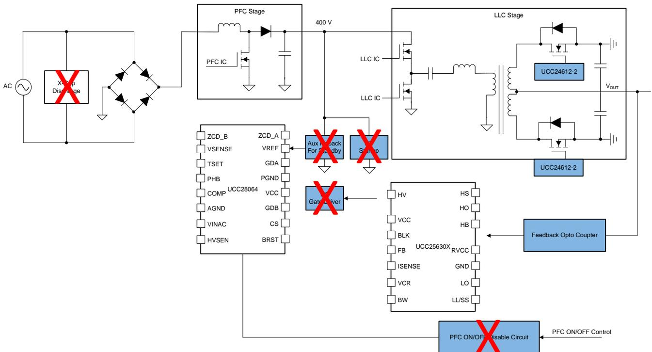
Figure 3. UCC28064A + UCC25630x Based AC/DC Solution for Low Standby Power
