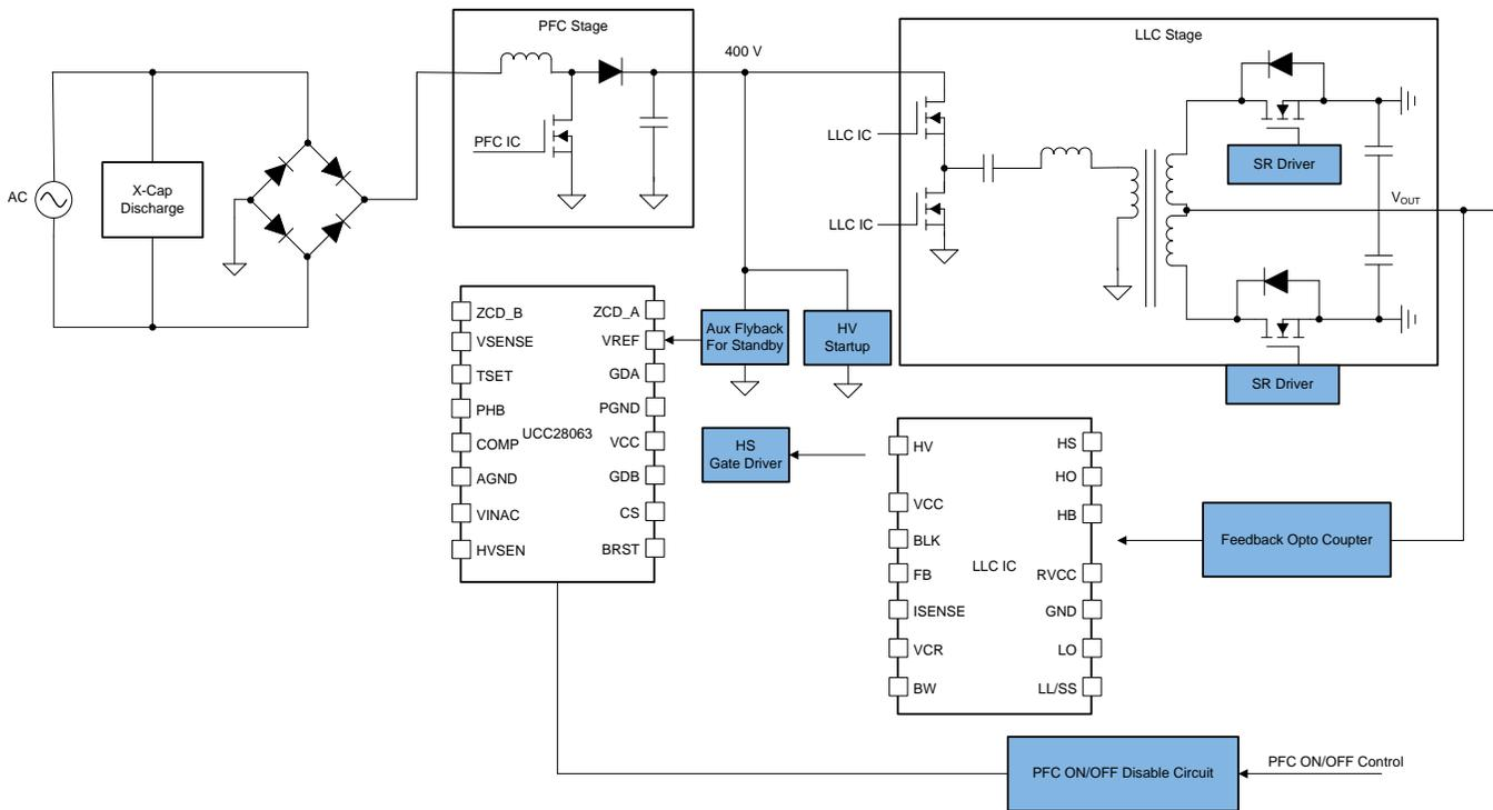
**Figure 1. UCC28063 + LLC IC Based AC-DC Solution for Low Standby Power**
