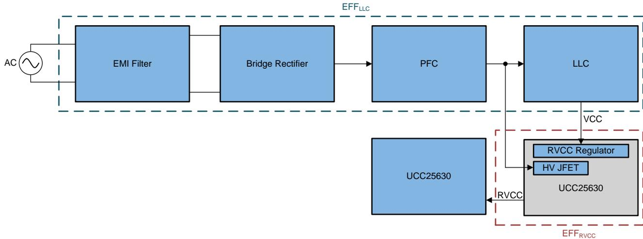
**Figure 10. VCC Generation Power Transfer Representation Along With Efficiency**
