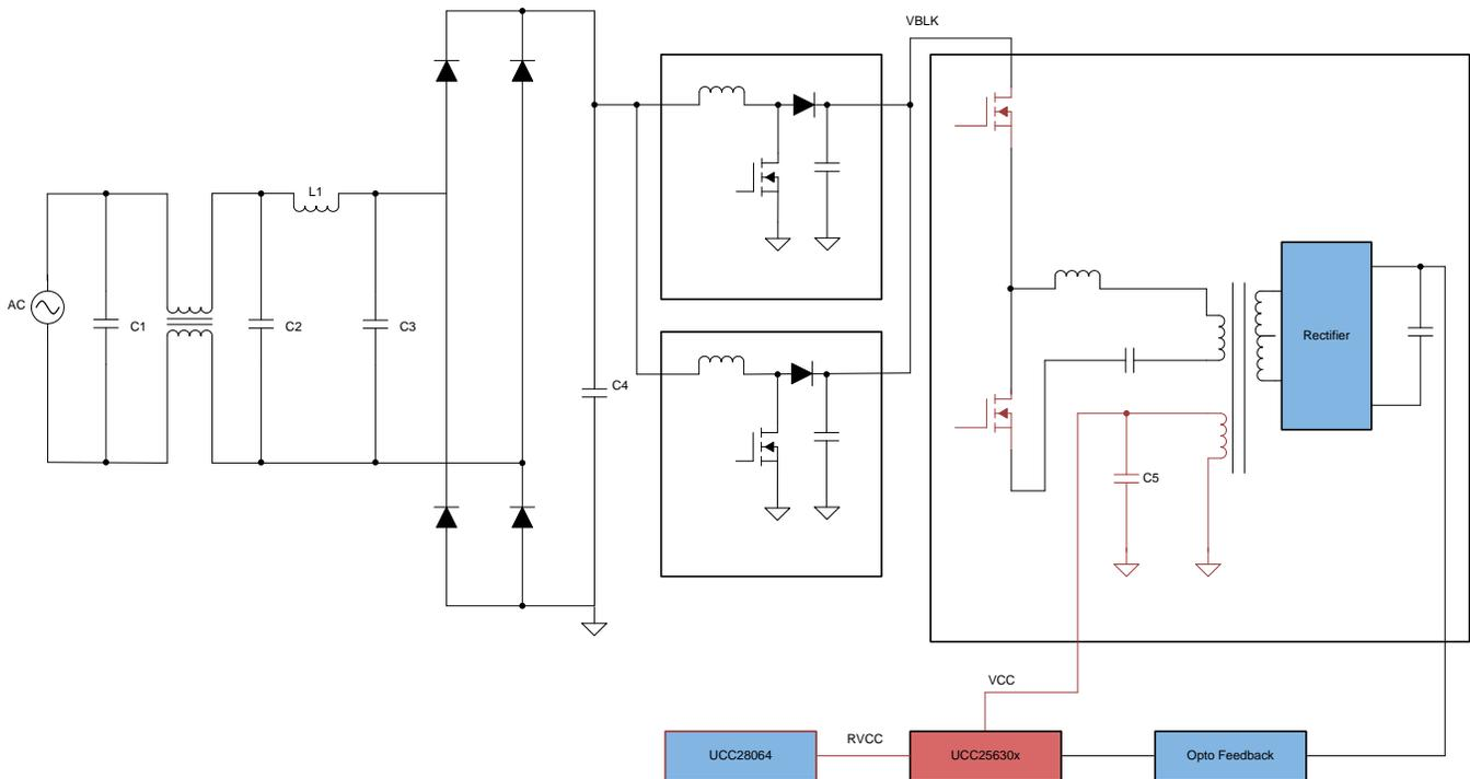
Figure 9. Power Transfer Model for RVCC Generation
