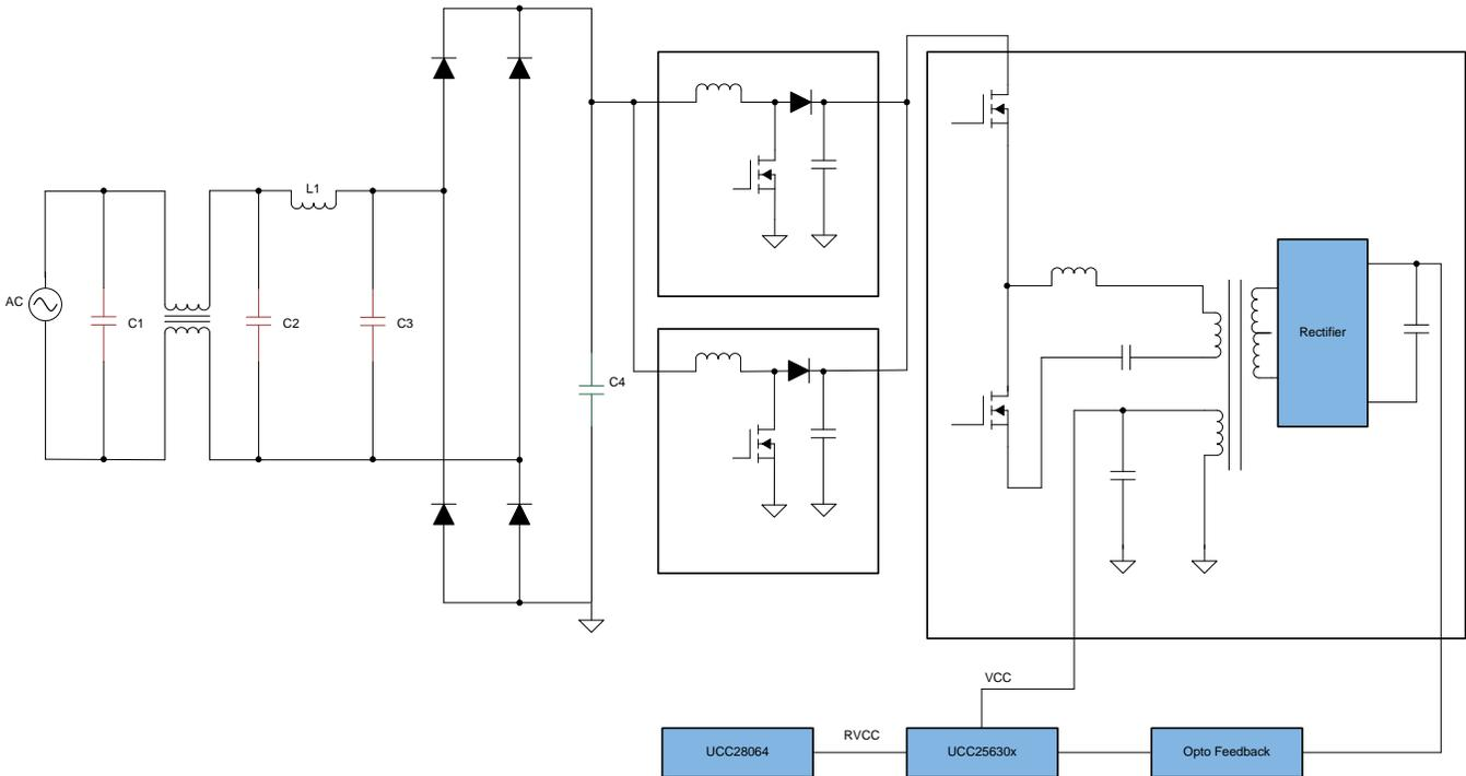
**Figure 5. AC/DC Power Supply With Interleaved Two-Phase PFC and LLC Converter Simplified Schematic**
