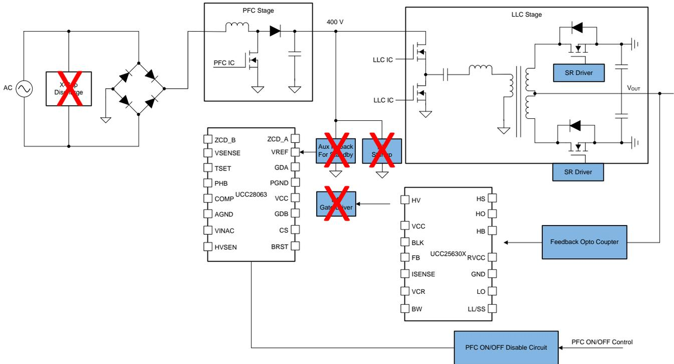
Figure 2. UCC28063 + UCC25630x Based AC-DC Solution for Low Standby Power
