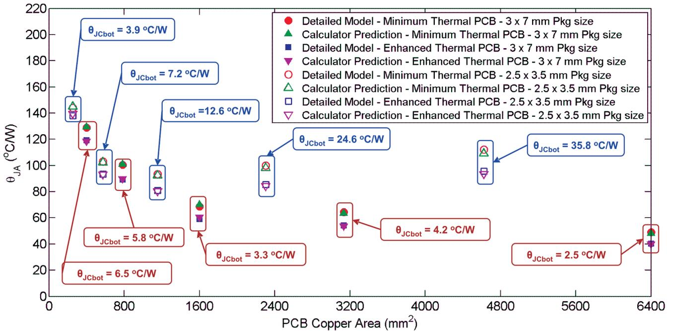
Figure 12. Validation of Interpolation Approach for Inline Packages
