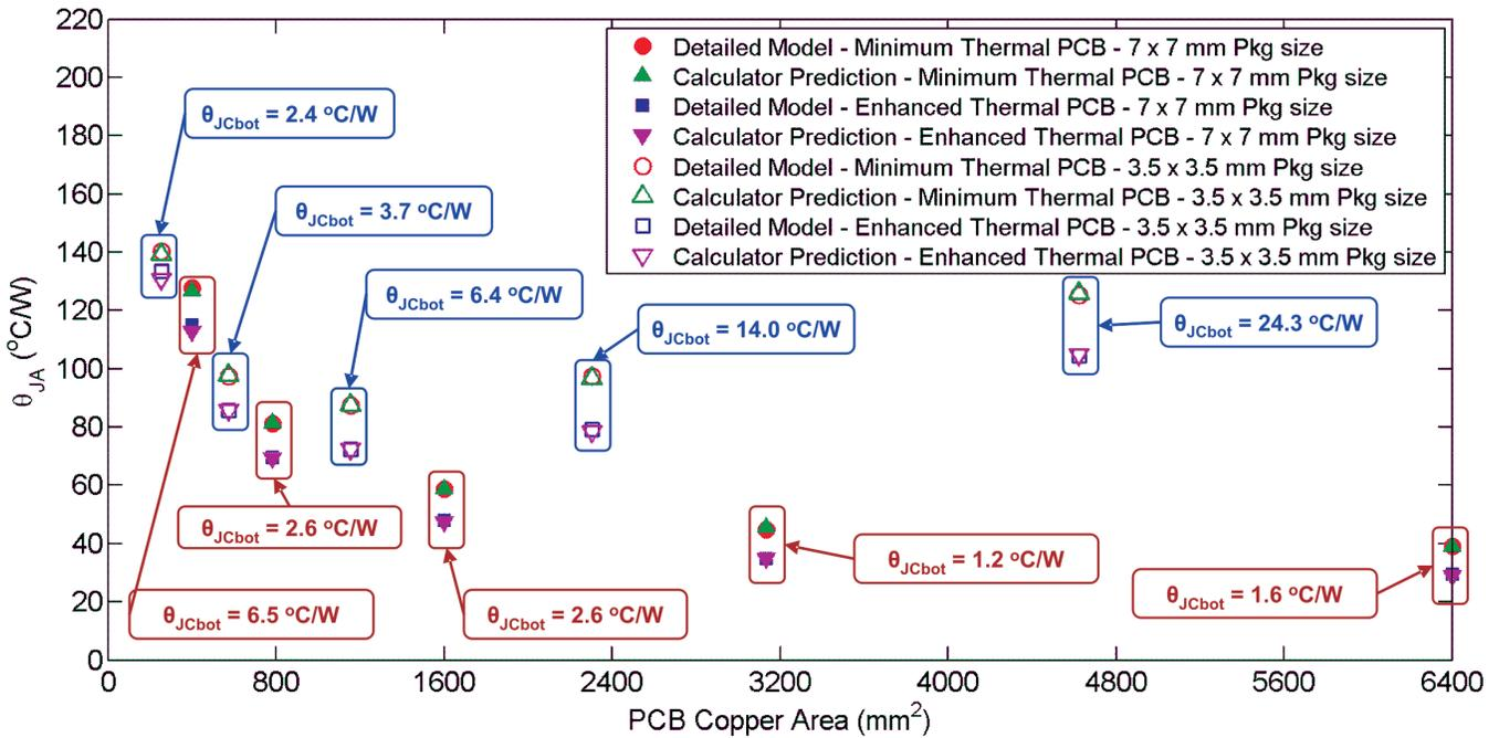
Figure 11. Validation of Interpolation Approach for Quad Packages
