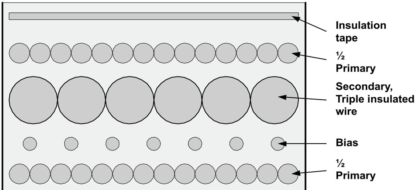
**Figure 4. Example of a Recommended Transformer Design.**
