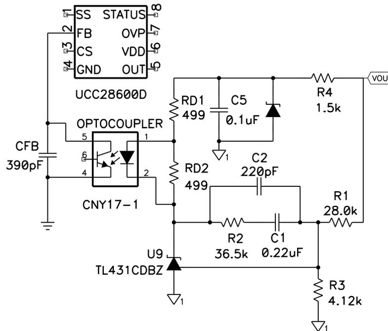
**Figure 8. Typical Loop Compensation for the UCC28600**
