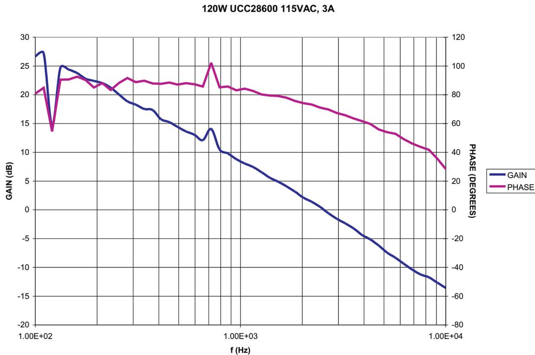
**Figure 9. Bode Plot for a 120-W Offline Converter**
