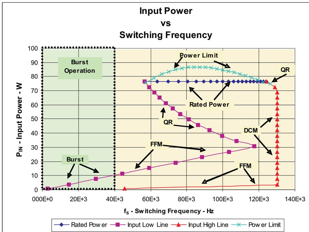
Figure 1. Boundaries with Respect to Input Power
