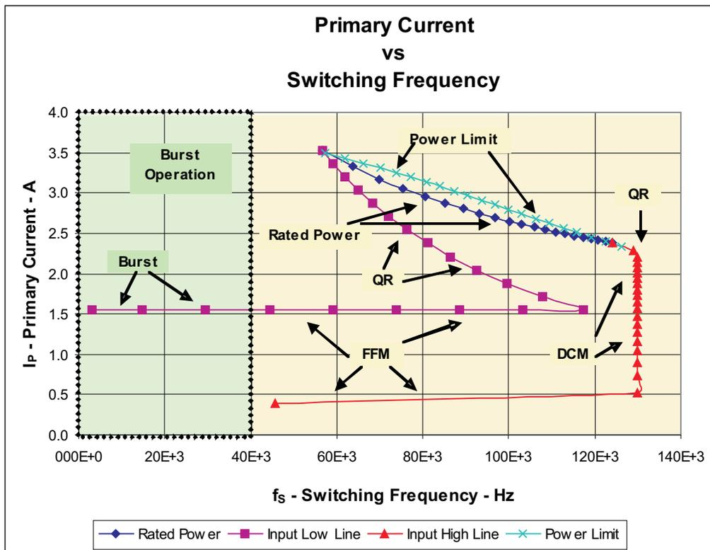
Figure 3. Boundaries with Respect to the Primary Current
