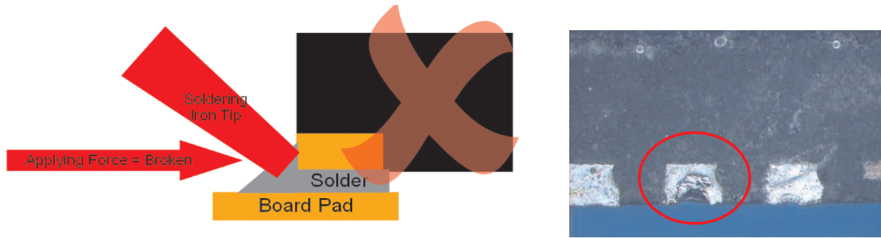
Figure 18. Manual Rework Damage
