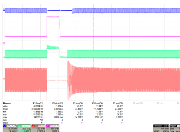
Figure 7. Overvoltage Protection After Injecting 45-V Pulses
