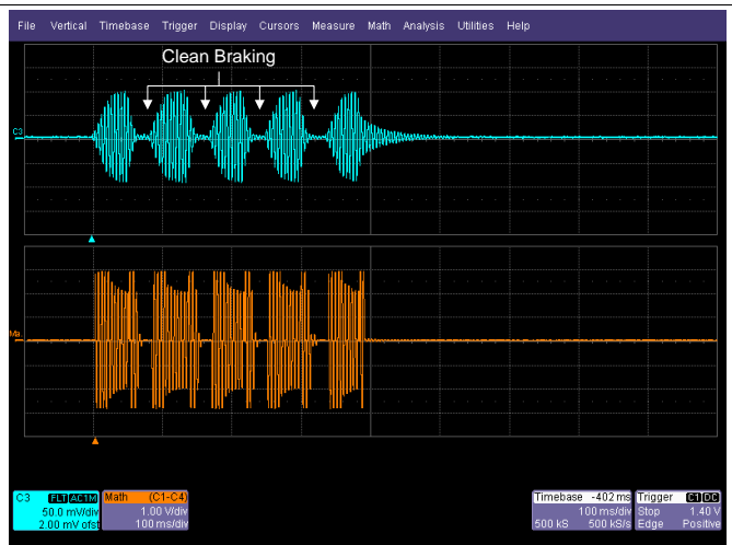
Figure 5. Pulsing Waveform in Closed-Loop
