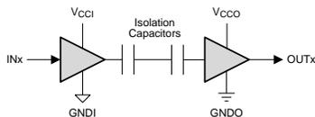
Figure 1. Series Capacitor Isolation
