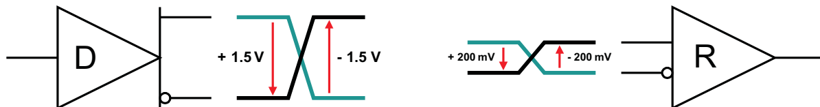
Figure 3. RS-485 Specified Minimum Bus Signal Levels
