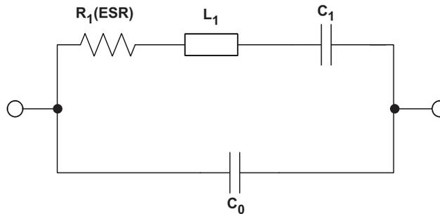
Figure 1. Equivalent Circuit of a Crystal
