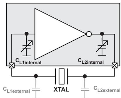
**Figure 2. Equivalent Circuit of the CDCE9xx Crystal Stage With Attached Crystal and External Load Capacitors**
