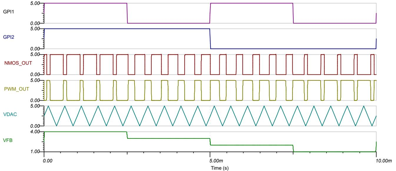
VS = 5 V, MARGIN\_HIGH\_CODE = 1023, MARGIN\_LOW\_CODE = 0, CODE\_STEP = 16, SLEW\_RATE = 4  $\mu$ s/step, MARGIN\_HIGH = 5 V, MARGIN\_LOW = 0 V, VDAC = 2-kHz triangle wave,  $R_1 = 5 \text{ k}\Omega$ ,  $R_2 = 2.5 \text{ k}\Omega$ ,  $R_3 = 5 \text{ k}\Omega$ ,  $R_4 = 5 \text{ k}\Omega$
