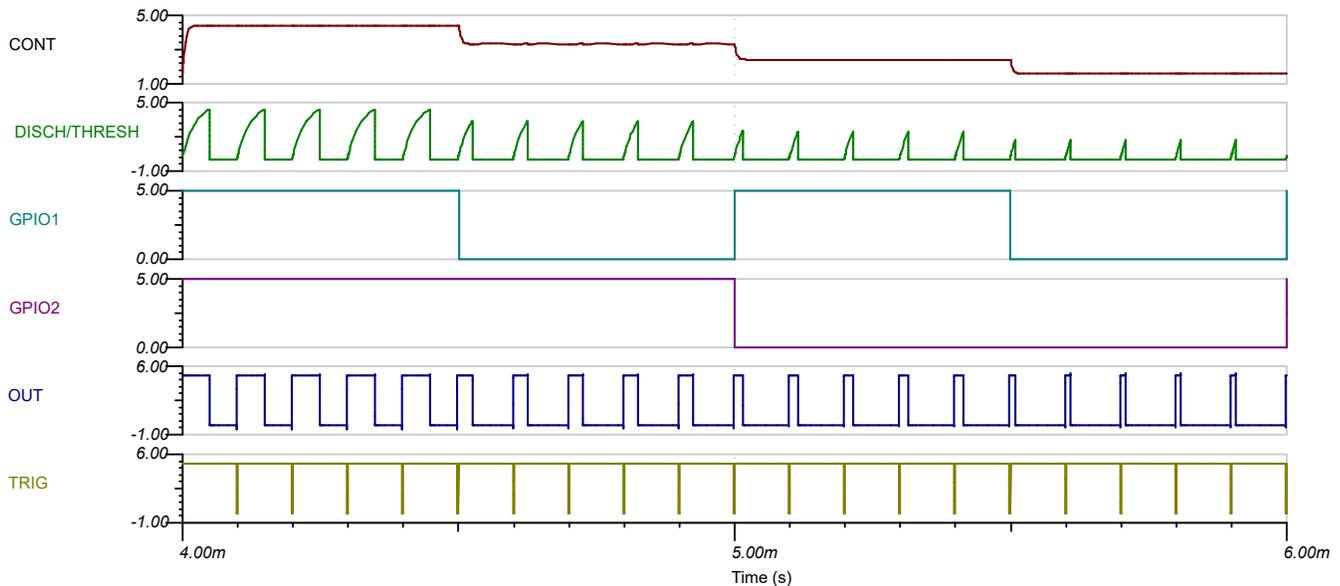
VS = 5 V,  $R_A = 12\text{ k}\Omega$ ,  $C = 2\text{ nF}$ , TRIG = 100-kHz square wave with 98% duty cycle,  $R_1 = 100\text{ k}\Omega$ ,  $R_2 = 50\text{ k}\Omega$
