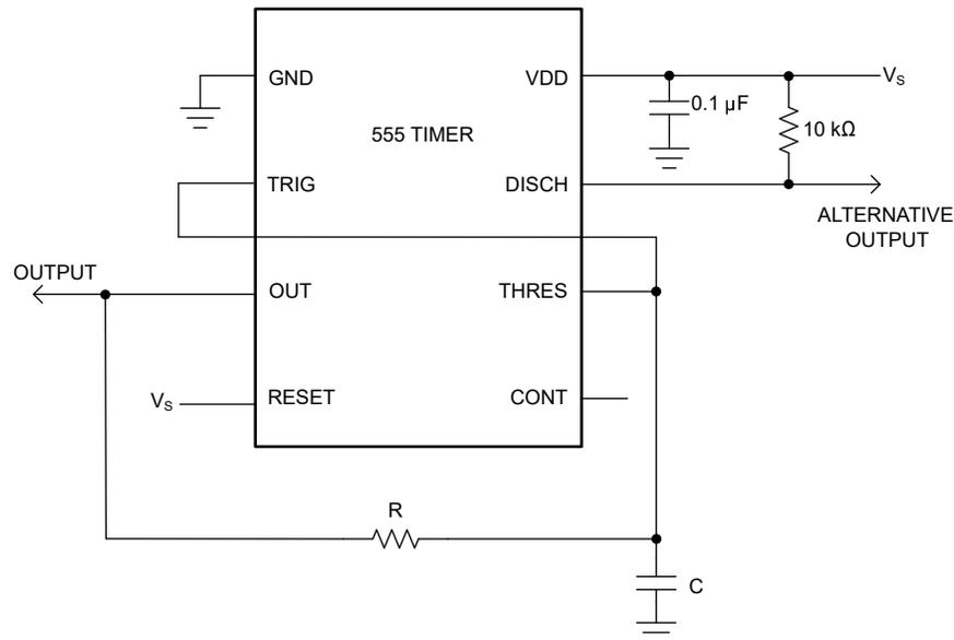
**Figure 3-1. 555 Timer Configured for a 50% Duty Cycle Oscillator**
