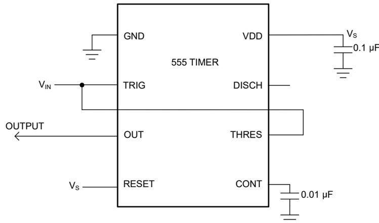
**Figure 6-1. 555 Timer Configured for a Comparator with Hysteresis**
