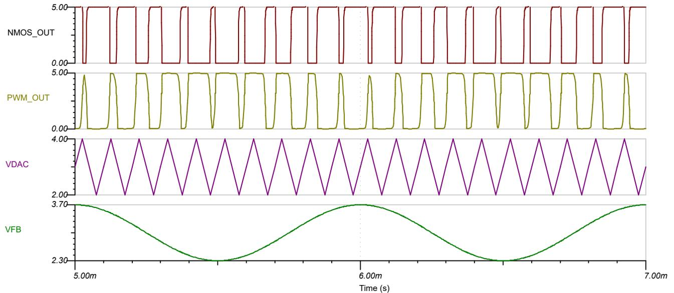
VS = 5 V, MARGIN\_HIGH\_CODE = 810, MARGIN\_LOW\_CODE = 410, CODE\_STEP = 32, SLEW\_RATE = 4  $\mu$ s/step, MARGIN\_HIGH = 4 V, MARGIN\_LOW = 2 V, VDAC = 10-kHz triangle wave, and VFB = 1.2-Vpp 1-kHz sine wave with a 3-V DC offset
