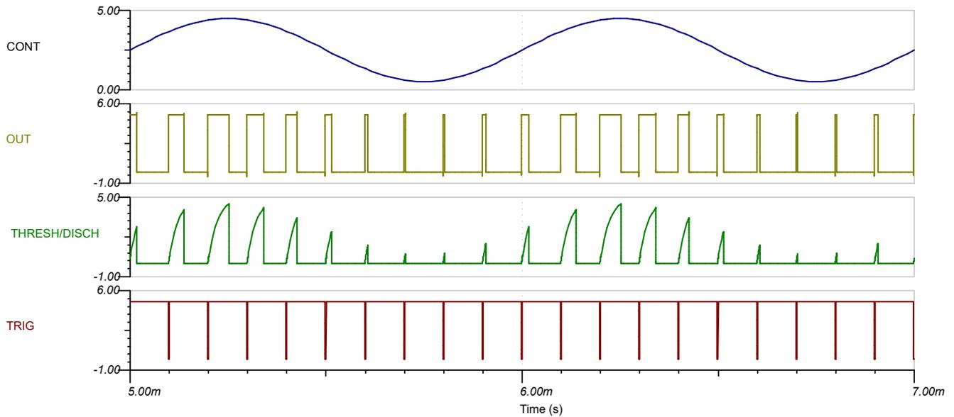
VS = 5 V, R<sub>A</sub> = 12 kΩ, C = 2 nF, TRIG = 100-kHz square wave with 98% duty cycle, and CONT = 4-V<sub>pp</sub> 1-kHz sine wave with a 2.5-V DC offset
