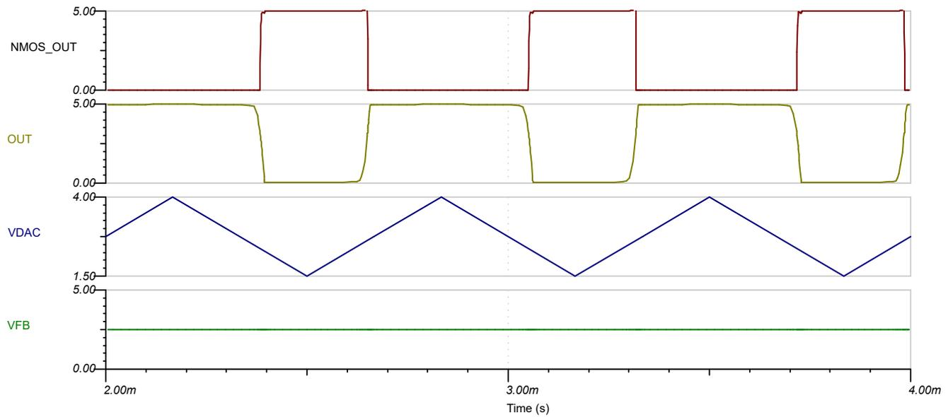
VS = 5 V, MARGIN\_HIGH\_CODE = 810, MARGIN\_LOW\_CODE = 310, CODE\_STEP = 32, SLEW\_RATE = 4  $\mu$ s/step, MARGIN\_HIGH = 4 V, MARGIN\_LOW = 1.5 V, VDAC = 1.5-kHz triangle wave, and VFB = 2.5 V
