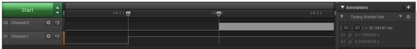
**Figure 4-1. First Power-on FLL Lock Time for MSP430FR2355 With the Fast Lock Code Example**
