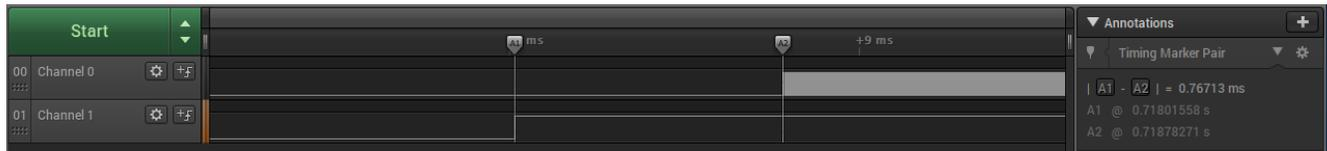
**Figure 3-2. FLL Lock Time on MSP430FR2355 LaunchPad™ Development Kit With the Fast Lock Code Example**
