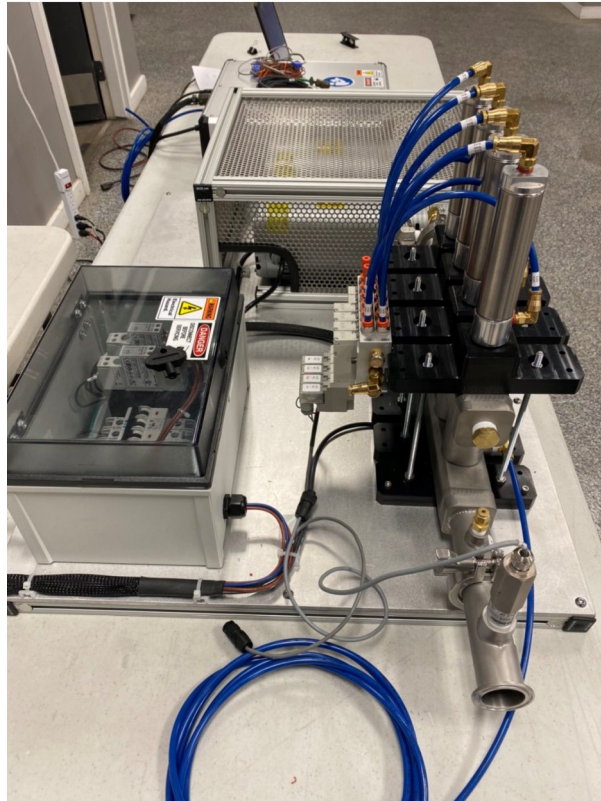
Figure 3-1. Sonic Nozzle Test and Calibration System
