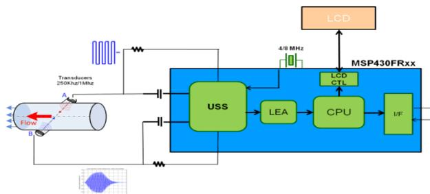
**Figure 1-2. Complete Leak Detection System**
