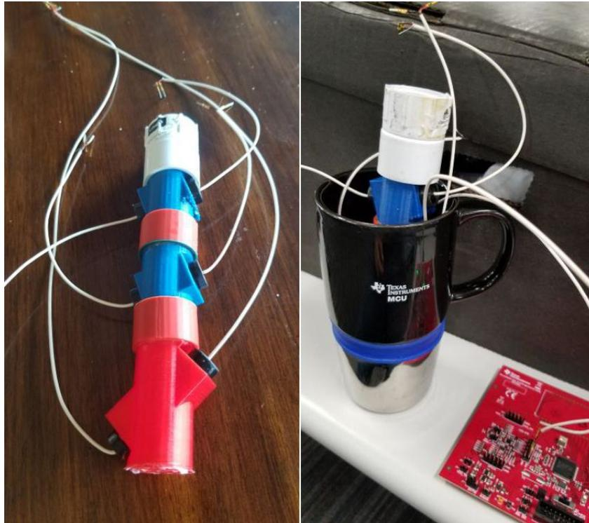
**Figure 2-1. 3D Printed Fixture and EVM**
