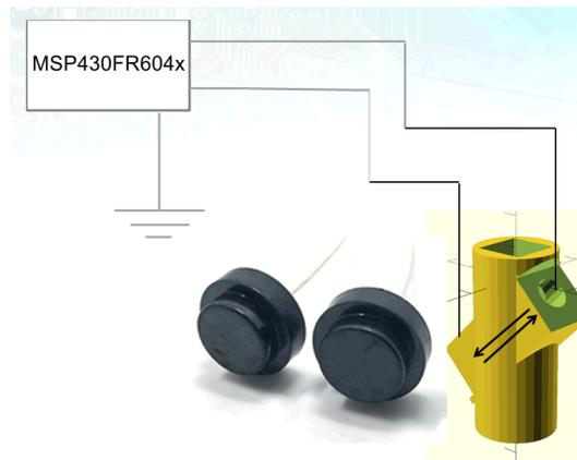
**Figure 2-2. Jiakang 2-MHz Ultrasonic Configuration**
