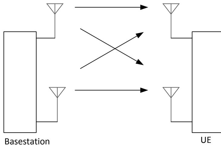
Figure 1. Single-User MIMO in LTE TM4
