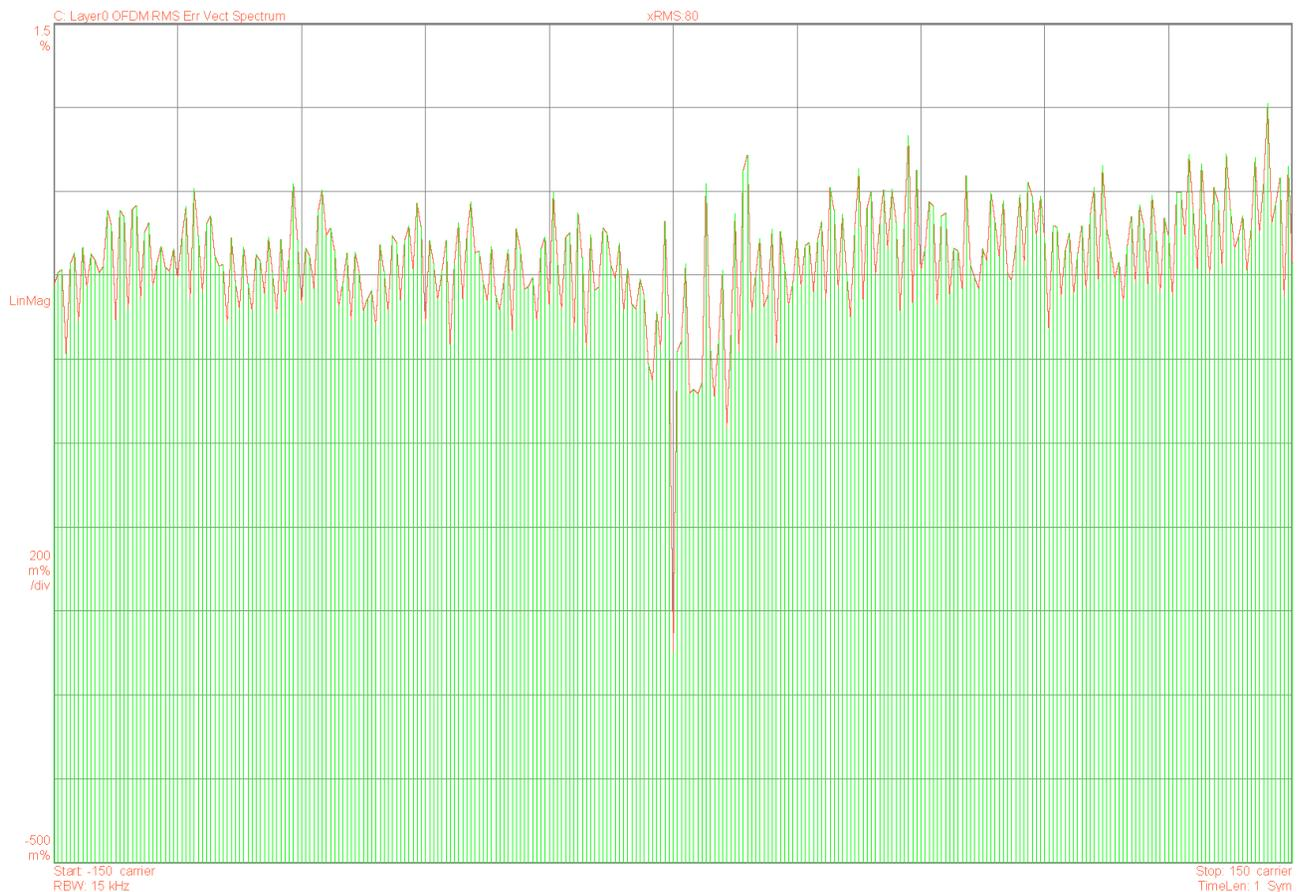
**Figure 10. RMS EVM vs Carrier Frequency for 1 OFDM Symbol**
