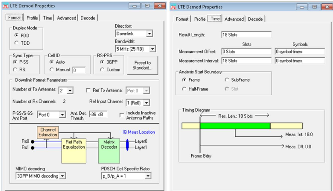
Figure 7. VSA Demodulation Settings for 5-MHz LTE 2x2 MIMO Waveform
