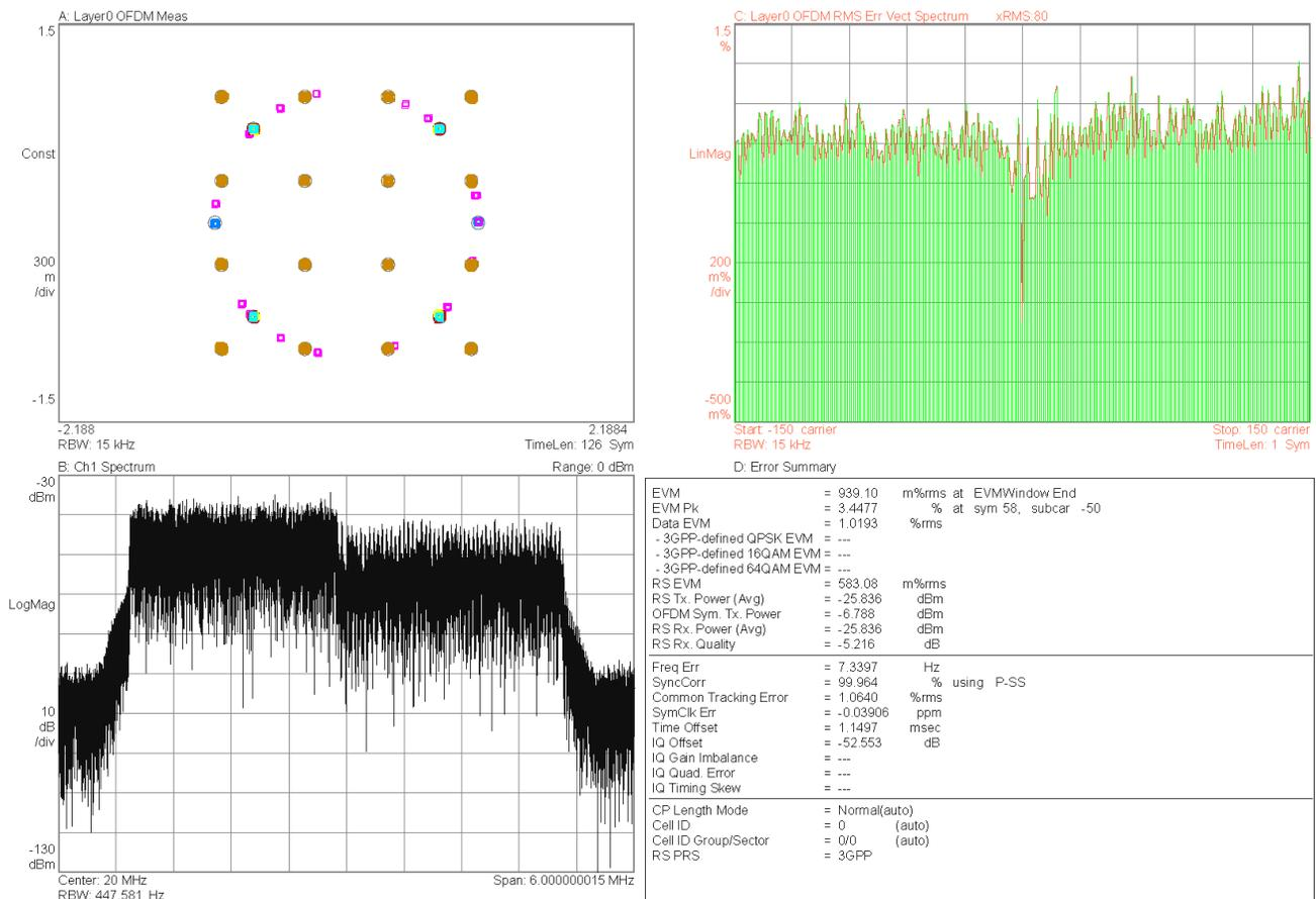
Figure 8. Constellation, Spectrum, EVM vs Carrier Frequency and Error Summary Results After Demodulation
