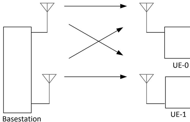
Figure 2. Multi-User MIMO in LTE TM5
