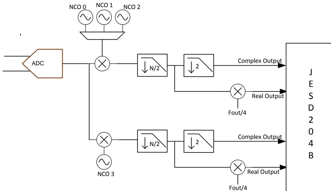
Figure 6. Receiver Data Path in AFE76xx
