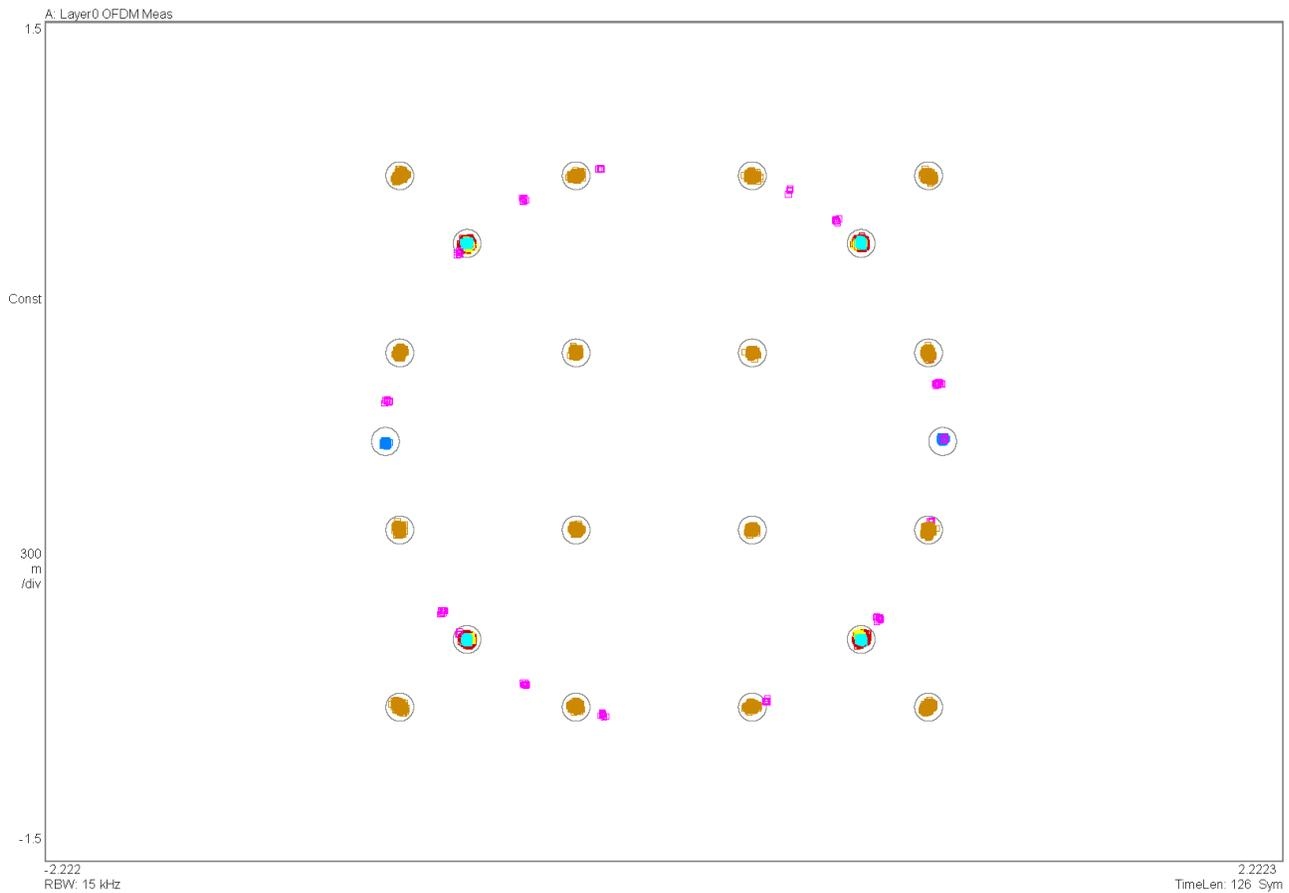
**Figure 9. Received Constellation of 5-MHz LTE 2x2 MU-MIMO Test Pattern**
