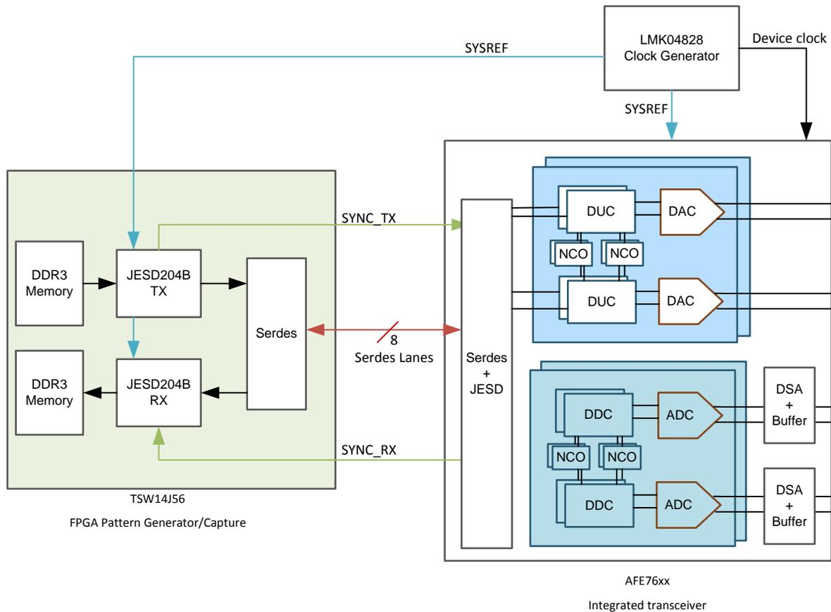
Figure 4. Block Diagram of 2x2 MIMO Transceiver
