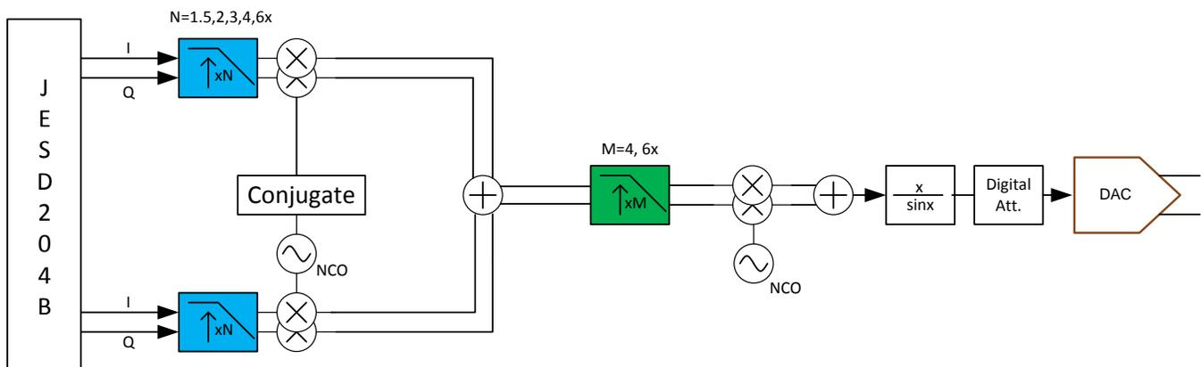
Figure 5. Transmitter Data Path in AFE76xx
