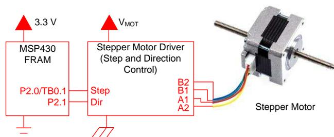
Figure 1. Stepper Motor Circuit Diagram
