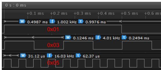
**Figure 2. Frequency Modulation**
