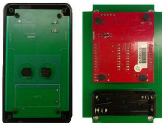
Figure 4. Top and Bottom View of the Grip Detection BoosterPack
