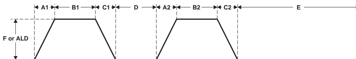
**Figure 1-3. Programming for Blink Modes and Intensity**
