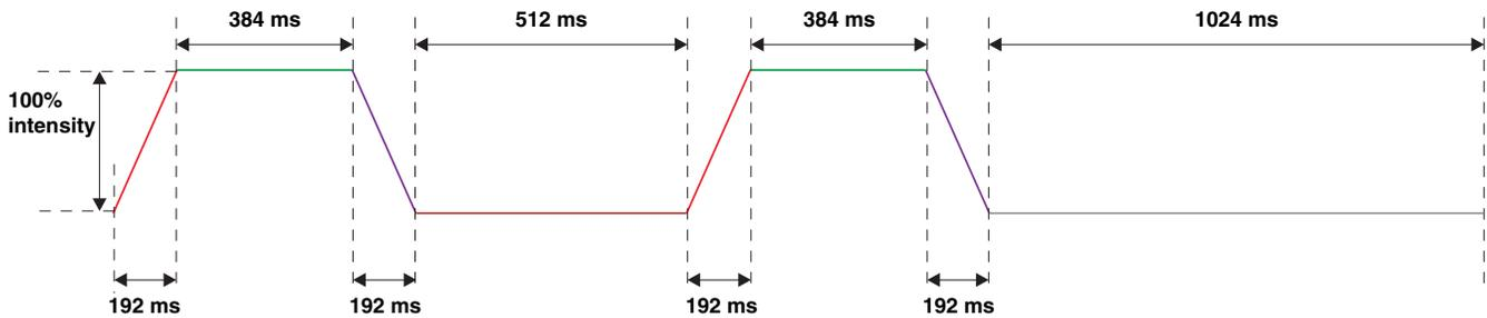
**Figure 1-4. LED Blink Cycle Example**
