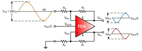
Figure 2. Attenuator Fully Differential Amplifier Configuration
