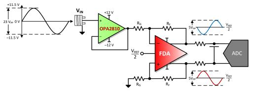
Figure 3. Hi-Z Signal Chain With an OPA2810 Buffer Stage
