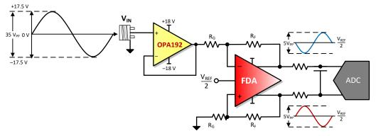
Figure 4. Hi-Z Signal Chain With an OPA192 Buffer Stage
