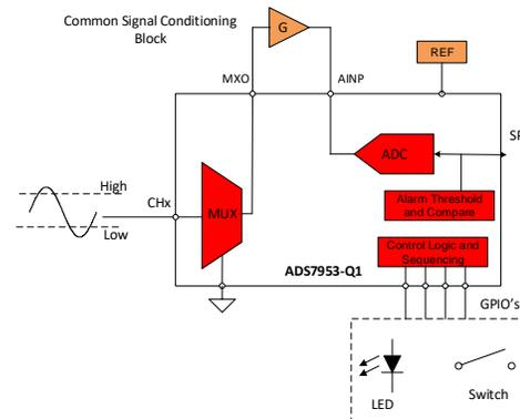
**Figure 4. Functional Block Diagram of ADS7953-Q1 Showing GPIO/ALARM Functionality**
