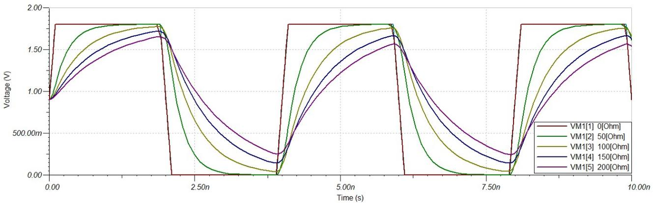
**Figure 3-6. 250 MHz CMOS output. Fixed 5 pF load, varying resistance.**
