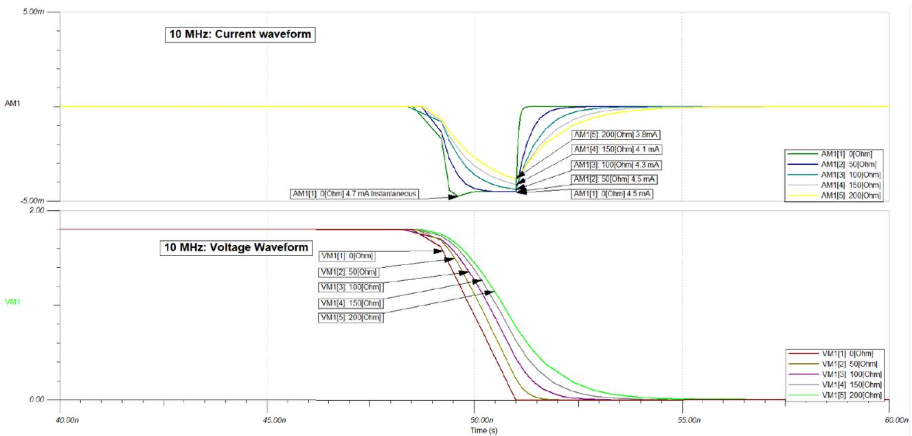
Figure 3-4. Zoom: Current and Voltage waveforms at 10 MHz. Fixed 5 pF load, varying resistance.
