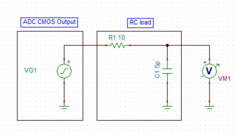
**Figure 3-1. Simple CMOS RC voltage model**
