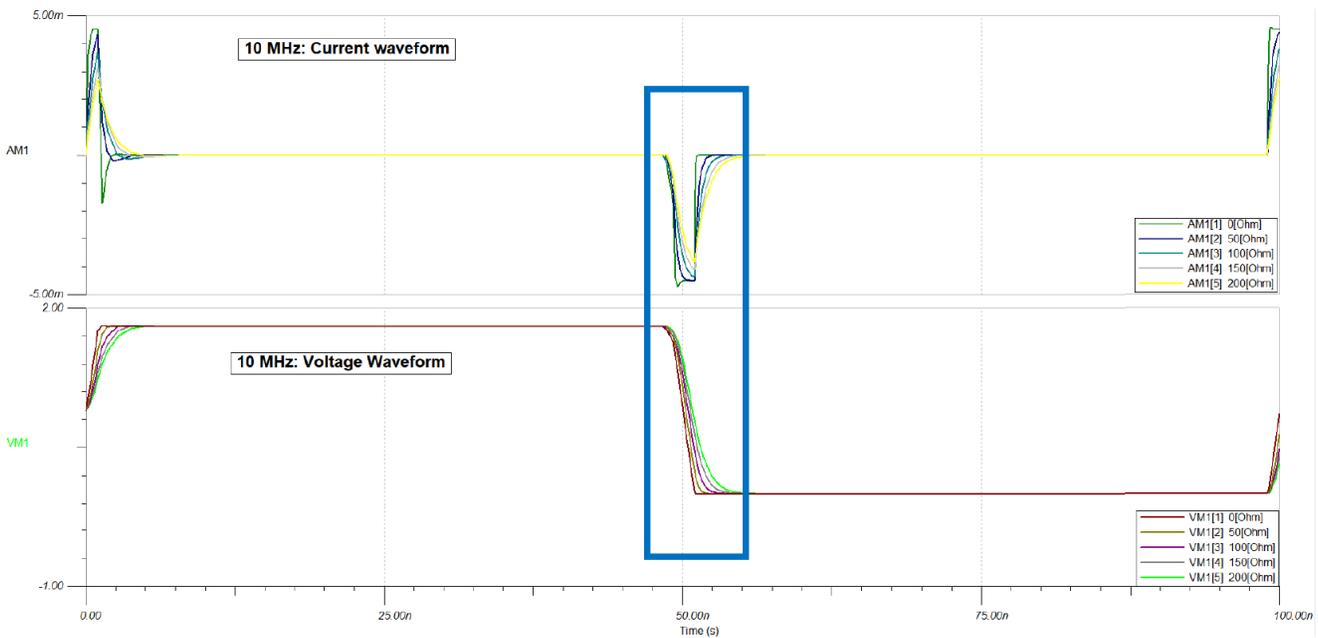
Figure 3-3. Current and Voltage waveforms at 10 MHz. Fixed 5 pF load, varying resistance.
