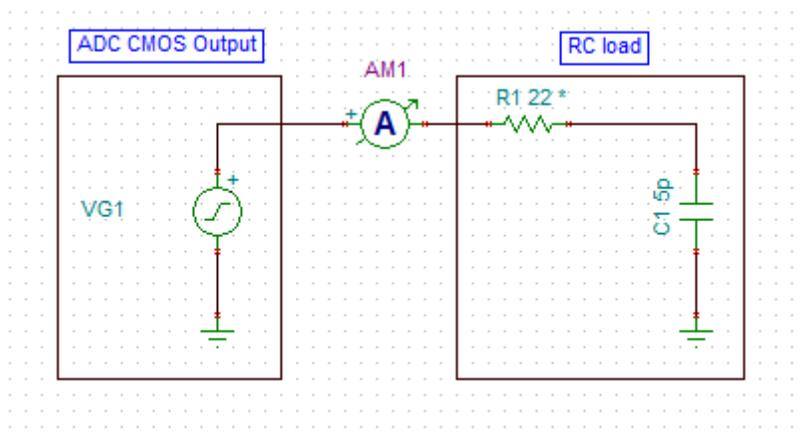
**Figure 3-2. Simple CMOS RC instantaneous current model**
