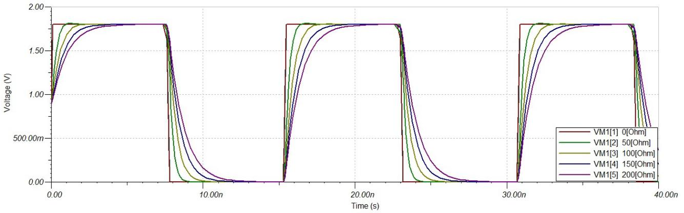
**Figure 3-5. 65 MHz CMOS Voltage Waveform. Fixed 5 pF load, varying resistance.**
