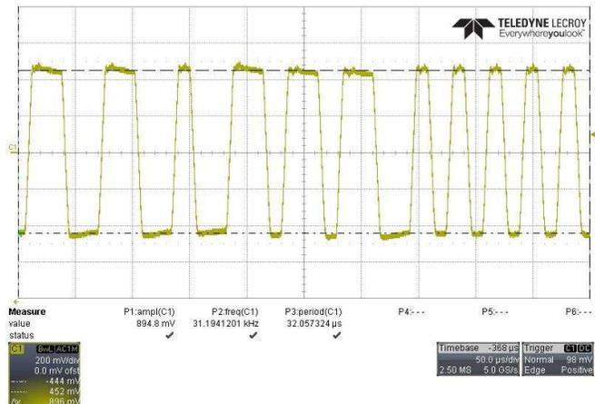
**Figure 3. Bus Voltage with FF/PA Signal Transmitted**
