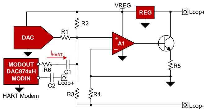
**Figure 2. HART Coupling in Loop Powered Transmitter**
