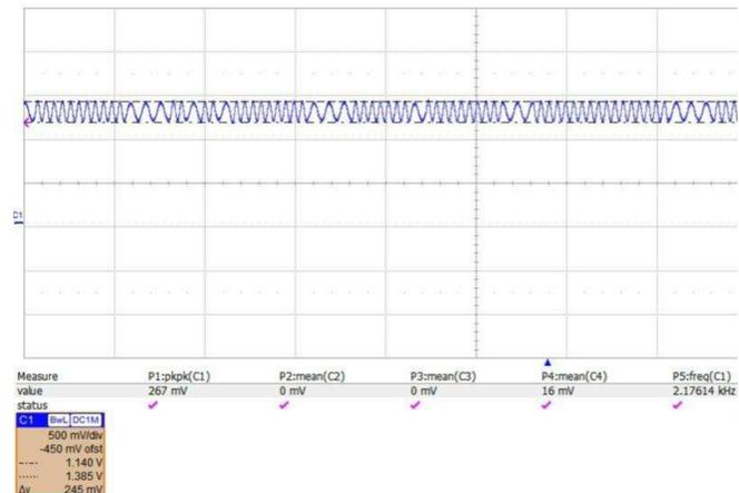
**Figure 3. 2-Wire Transmitter DC Value with HART**
