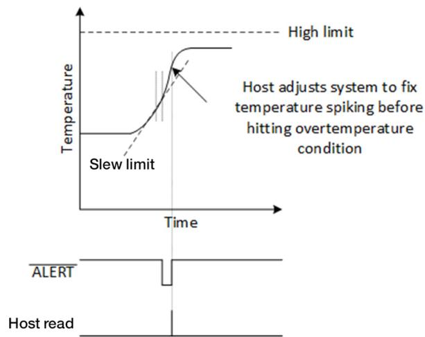
**Figure 3. The New Slew-rate Alert Feature in the TMP126**
