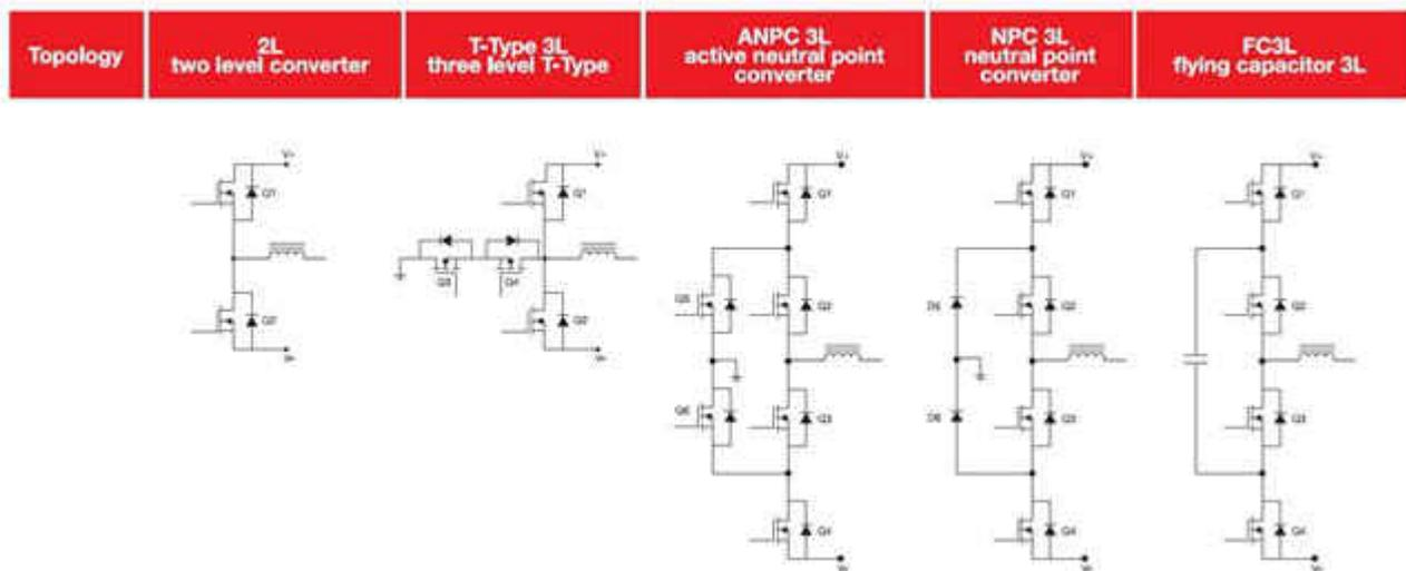
**Figure 3. Power Topologies for Half-bridge and Branch Equivalent**
