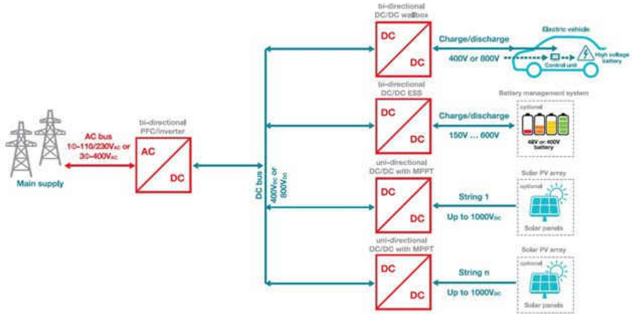
**Figure 2. A Typical Solar Inverter System With an Energy Storage System**
