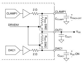
Figure 6-1. AFE10004 Output Switches
