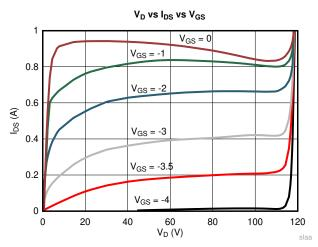
Figure 1-2. FET V<sub>D</sub>, I<sub>DS</sub>, and V<sub>GS</sub> Behavior
