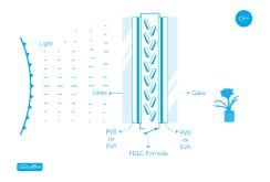
Figure 2-1. PDLC Film in the Off State (no applied voltage)
