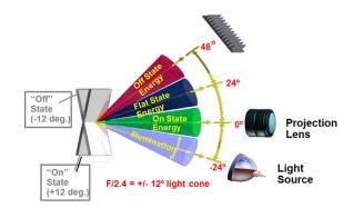
Figure 3-1. Illumination Diagram of Standard DLP Projector
