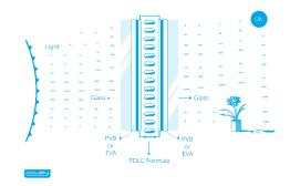
Figure 2-2. PDLC Film in the On State (+48V applied)
