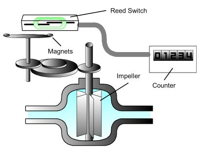
Figure 4. Electromagnetic Pulse Measure Principle
