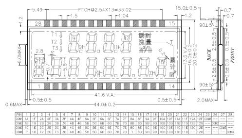
Figure 12. LCD Specification
