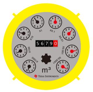
Figure 1. Mechanical Water Meter Dial
