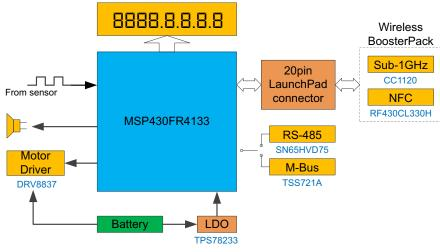
Figure 7. Block Diagram
